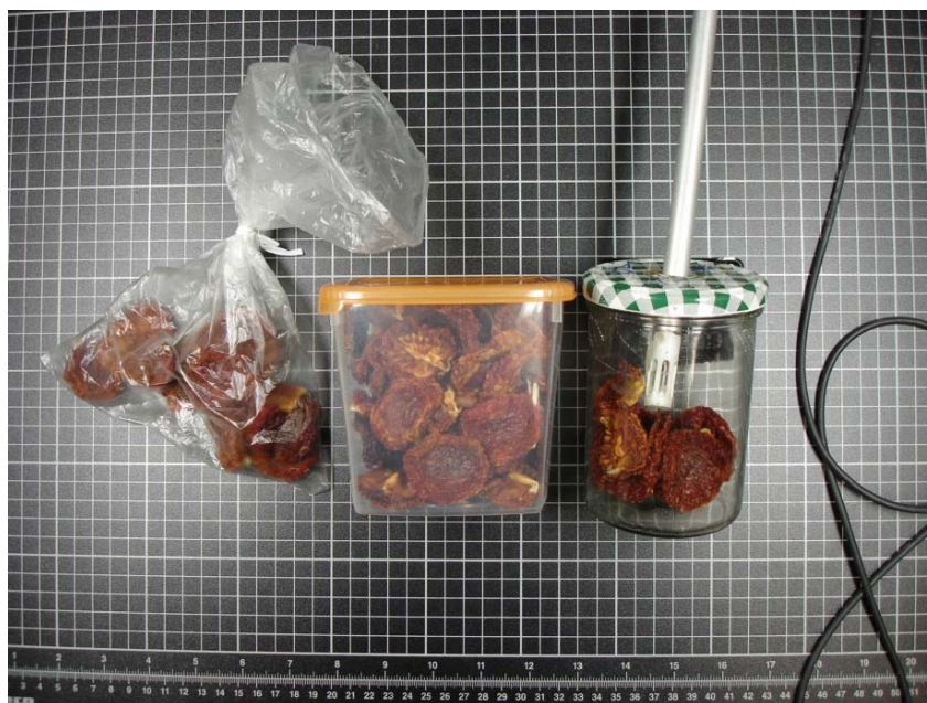
Figure 5.1: Storage containers with samples; left: PE bag, middle: plastic jar, right: glass jar with temperature/rH sensor
