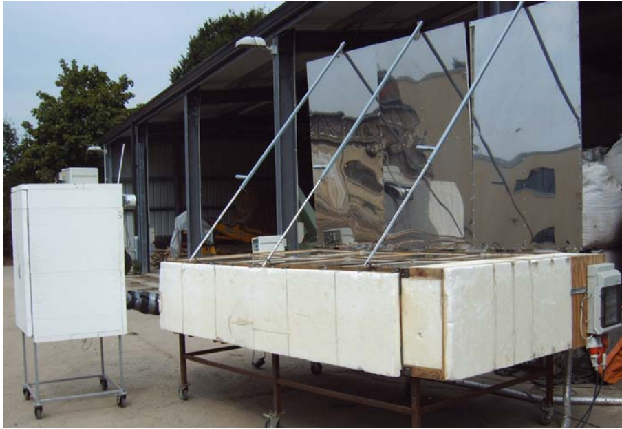
Figure 3.4: Photograph of solar collector and drier in operation
