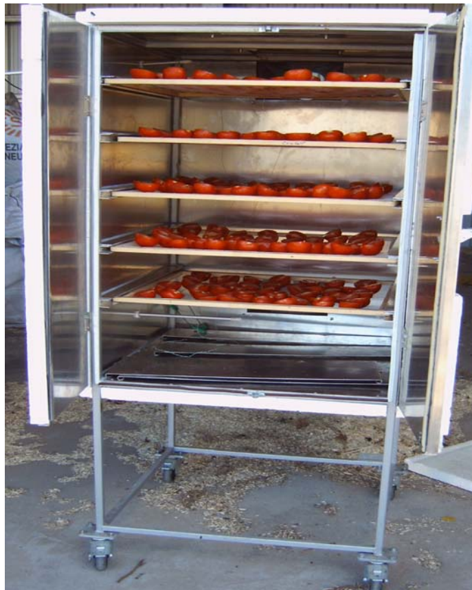
Figure 3.5: Photograph of solar drier loaded with tomato for drying
