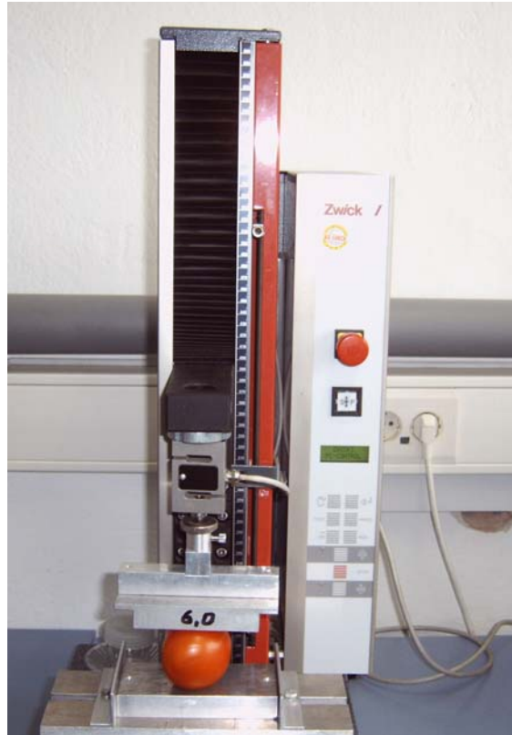
Figure 1.8: Compression tests of tomato using a 'Zwick' Universal Testing Machine
