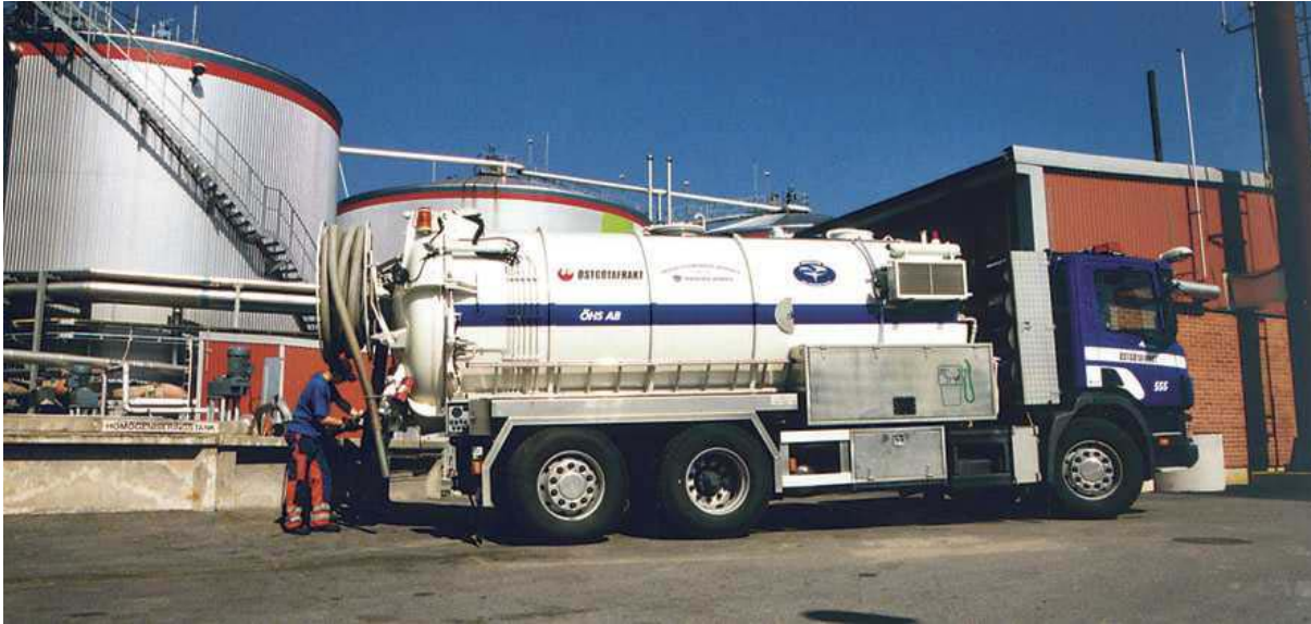
Fig. 4. Unloading of organic material from the first biogas driven industrial vacuum truck.
