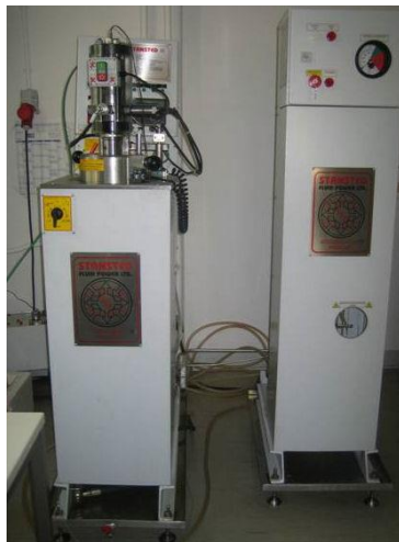
Figure 2. 12. Stansted Mini Foodlab FBG5620 high pressure unit with pressure temperature profile measured inside the pressure vessel. Adapted from Mathys (2008a).
