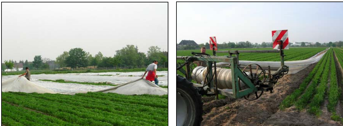
Figure 2: As soon as temperatures permit, the fleeces or films are folded up by hand (left). The subsequent mechanical rolling up of the fleeces or films is performed from the edge of the bed, and is supervised by two workers (right)
