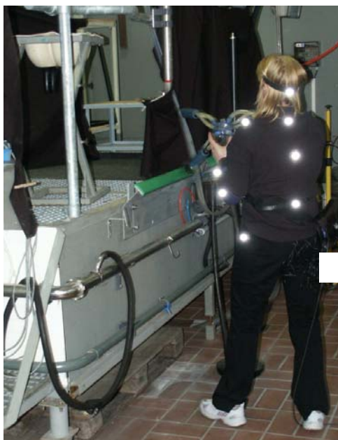
Figure 1: Experimental setting working height above shoulder level with light milking unit showing the marker positions
