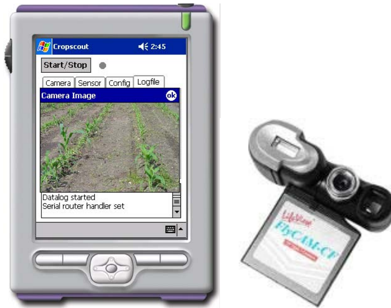
Figure 8: iPAQ Pocket PC providing the graphical user interface and running the image processing (row recognition). As imaging device a compact flash camera is used.
