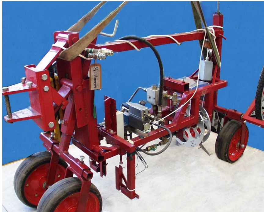
Fig. 9: The mechanical weed control device for field experiments
