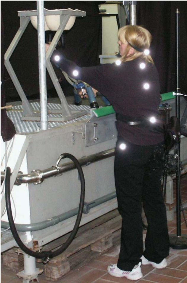
Figure 1: Location of markers, working height above shoulder level, conventional cluster
