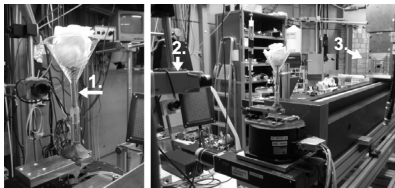
Figure 1: Experimental set up at BAM-Line, BESSY. 1. Sample container filled with water to prevent drying. 2. CCD camera for chlorophyll fluorescence imaging device. 3. CCD camera for x-ray imaging located 1.1 meter downstream of the sample (phase-contrast mode).
