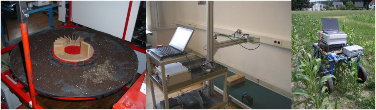
Figure 8: Experimental rigs (Rotating table, conveyor belt and test carriage for outdoor measurements)
