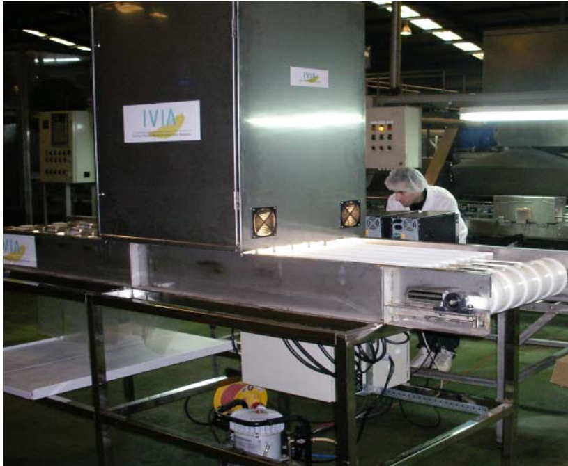
Figure 1: Prototype developed for the sorting of pomegranate arils
