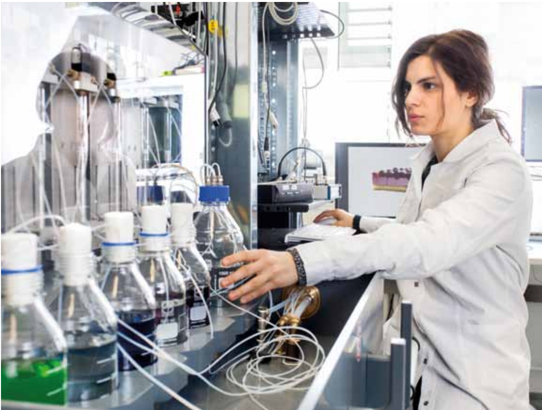
Figure 3: Exterior view of the computer-controlled gustometer – a device that delivers tastants to human observers for the study of taste perception. This high-precision device dispenses minuscule amounts of taste solutions.
