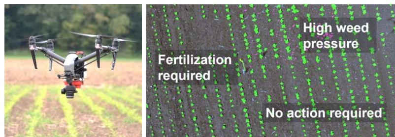
Figure 1. Left: UAV system (DJI Inspire II). Right: Sugar beet field in early season analyzed with our approach. We estimate the spatial distribution of crop (green) and weed (purple) and the per-plant canopy cover. This information directly leads to concrete suggestions for the farmers.
