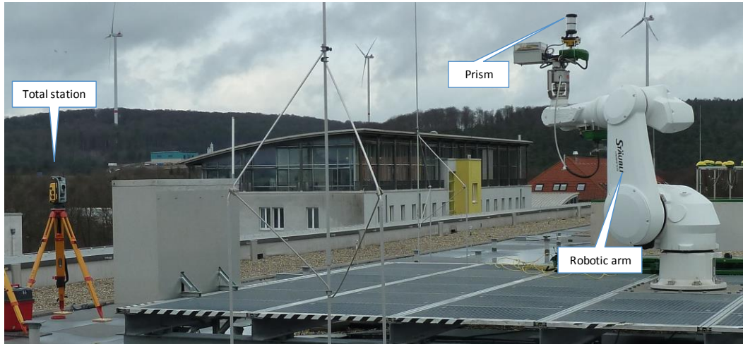
Figure 1: The total station that was used to track a prism on a robotic arm (photo: John Deere GmbH & Co. KG, Intelligent Solutions Group, Advanced Engineering, modified).
