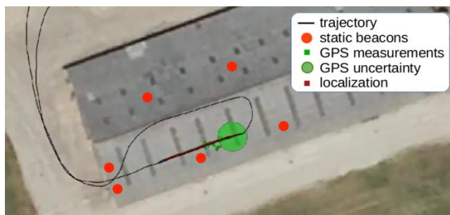
Figure 8: The trajectory of the robot and the position of the static beacons. The localization algorithm is running and the robot is in the barn
