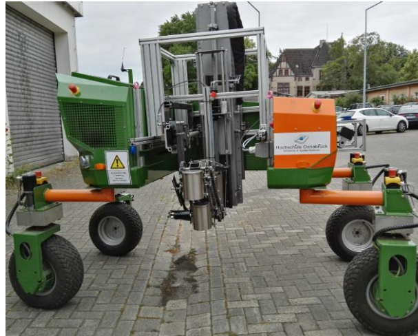
Figure 1: Autonomous field-robot BoniRob with "soil2data" application module
