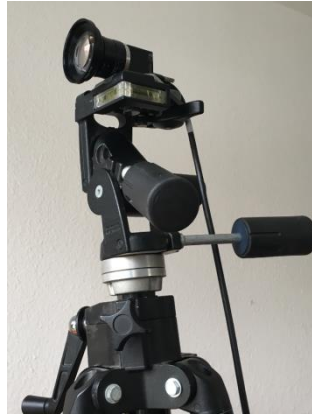
Figure 2: The image acquisition unit: a camera (Ximea-MQ042CG-CM), a wide-angle lens (AZURE-06520ML5M) and a tripod (Manfrotto-074B)
