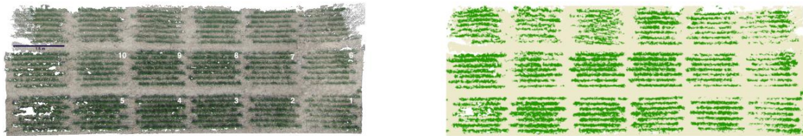
Figure 3: Left: Dense point cloud of a winter wheat genotype trial generated from aerial images using Pix4Dmapper by Pix4D. The numbers indicate the plot indices used for referencing. Right: Segmented point cloud generated using automated thresholding based on the excess green index and Otsu's method. Green points represent winter wheat and pale brown represents background.
