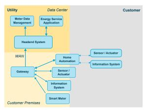
Figure 1: Traditional model for the Advanced Metering Infrastrucure. The utility's area of responsibility is depicted on the left, the customer's on the right. In some components (e. g. home automation, sensors and actuators), the sphere of influence overlaps or depends on the service model.
