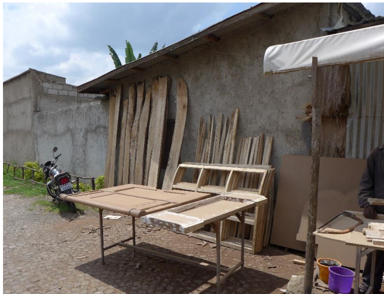
Figure 17: A small-scale furniture enterprise in Hawassa drying wood in the sun before processing Depending on the product, other inputs were required, such as MDF, paints, varnish, nails, glue, metal components, handles, leather or textiles. The wood used for the production of furniture originated from tree species indicated in the graph below.
