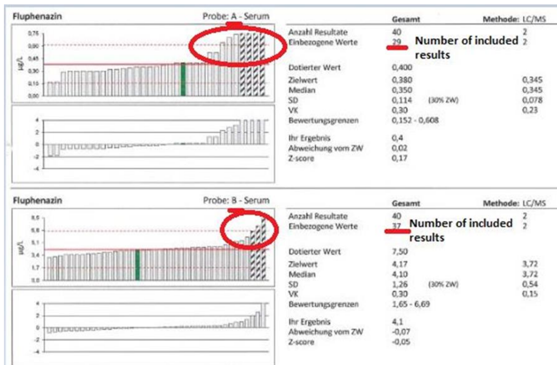
Figure 32 Results of the Round Robin Test for Fluphenazine, values higher than allowed circled in red, number of results included for sample B much higher than for sample A (Society of toxicological and forensic chemistry)
