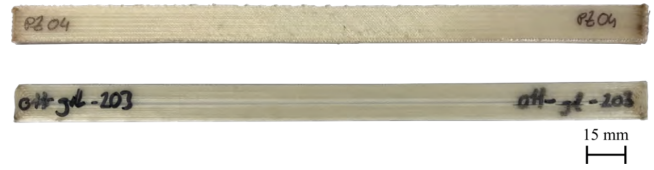
Fig. 7. the investigated tensile test specimens according to DIN EN ISO 527-5 [8] in Typ A orientation with different fill algorithm. Top: FullFiber , Bottom: Concentric .
