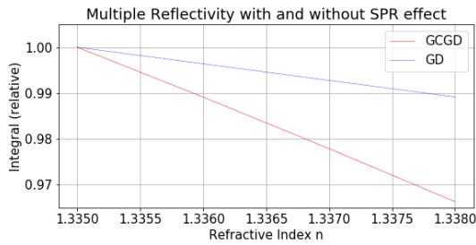
Fig. 6. Integral over multiple reflectivity depending on the refractive index of the analyte for two different interfaces.
