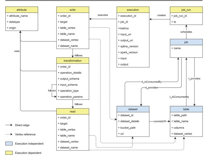
Fig. 3 Data model for the storage of Spark-based data lineage
