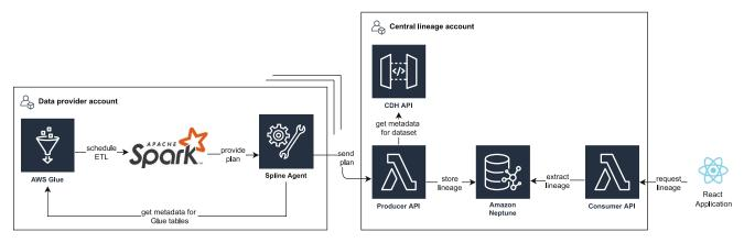
Fig. 2 Architecture of the implemented lineage tool
