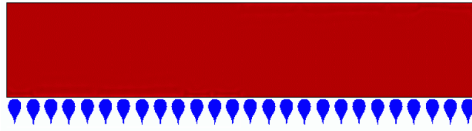
Figure 2: One-sided cooling of a hot slab.
