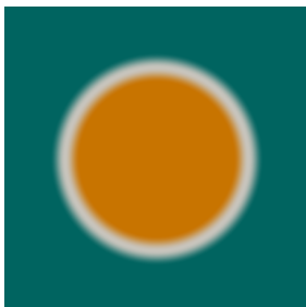
FIGURE 1. Initial phase field: A circular solid phase (orange) in a liquid environment (teal).
