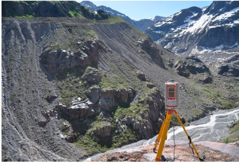
Figure 3. Light detection and ranging (LiDAR) point cloud acquisition of the test sites (G1/G2) using the TLS VZ-4000 (25 June 2019).
