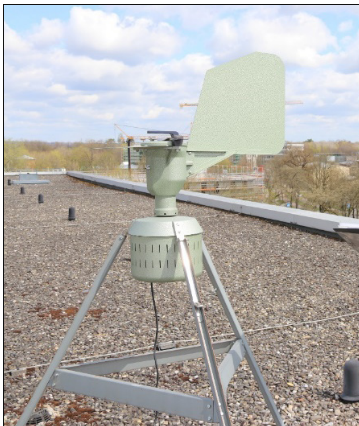
Fig. 3 7-day volumetric sampler.
