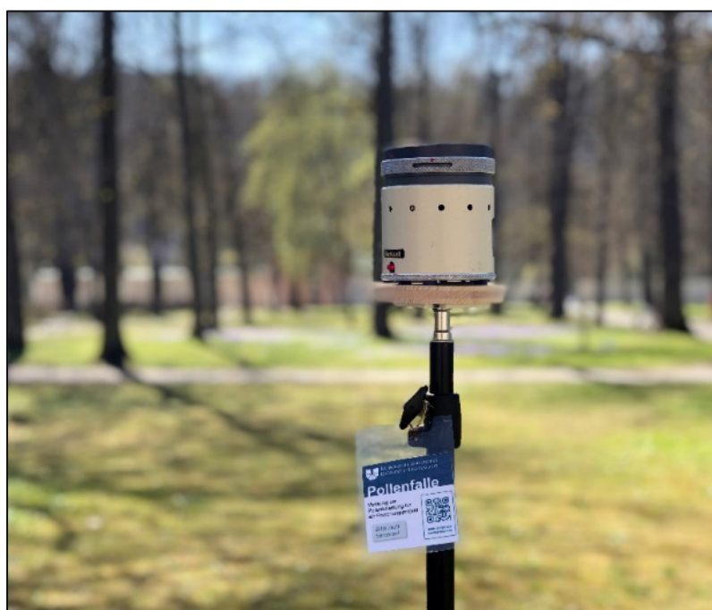
Fig. 4 Portable volumetric trap, mounted on a tripod at a height of 1.5 m.
