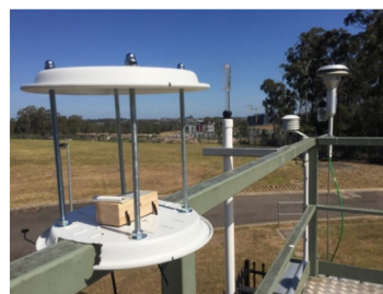
Fig. 3 Passive sampler mounted to the railing of an air quality monitoring station in Rouse Hill
