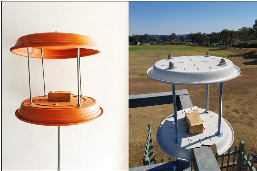
Fig. 5 Gravimetric pollen trap used in Germany (left) and Australia (right).
