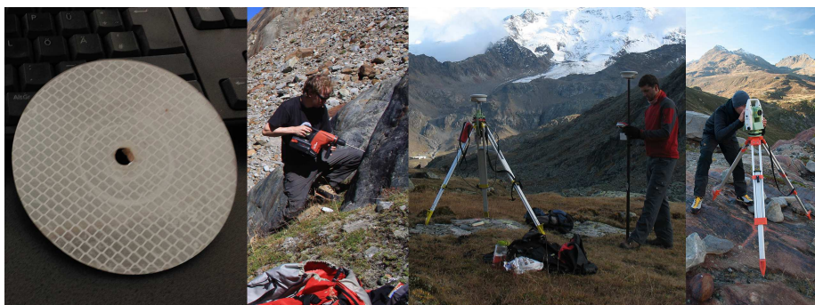
Figure 5.4.6: Reflector discs with a diameter of 10 cm (left) were fixed to non-moveable objects (2nd from left) and used for a better registration and georeferencing of TLS point clouds. These reflector discs were later surveyed exactly using a differential GPS device (2nd from right) and a total station (right).
