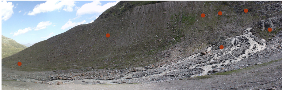
Figure 5.4.7: Reflector discs were placed at different distances and angles from the TLS scan positions. This image shows the location of reflector discs at scan position 16.
