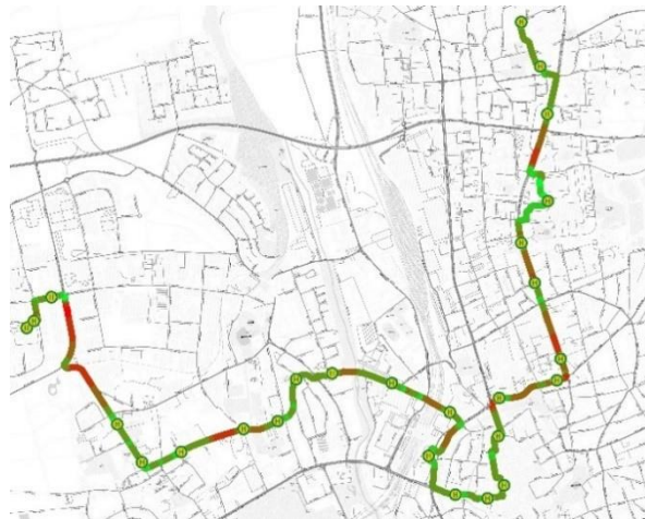
Figure 75. Analyzed bus line with the color indicating the vehicle speed. Left: Speed profile from SUMO simulation. Right: Speed profile from the actual bus
