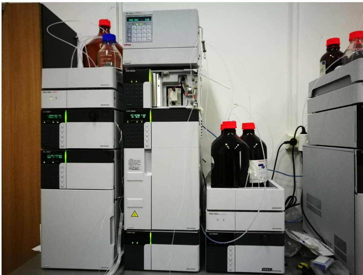
Figure 21. The HPLC-DAD-FLD setup used for the 4-ethylphenol analyses, Oenology Laboratory Iași, Romania
