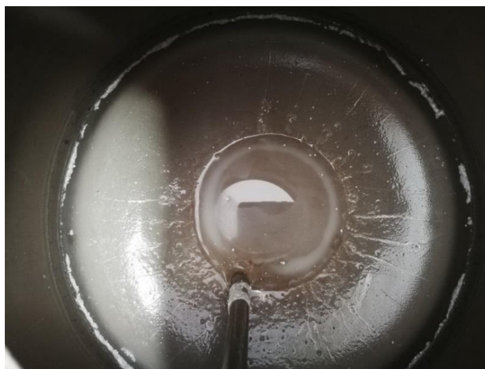
Figure 54. The aspect of the pressurized container after 4.15 g MIP2 suspended in 3 L water are pushed through the filter sheet
