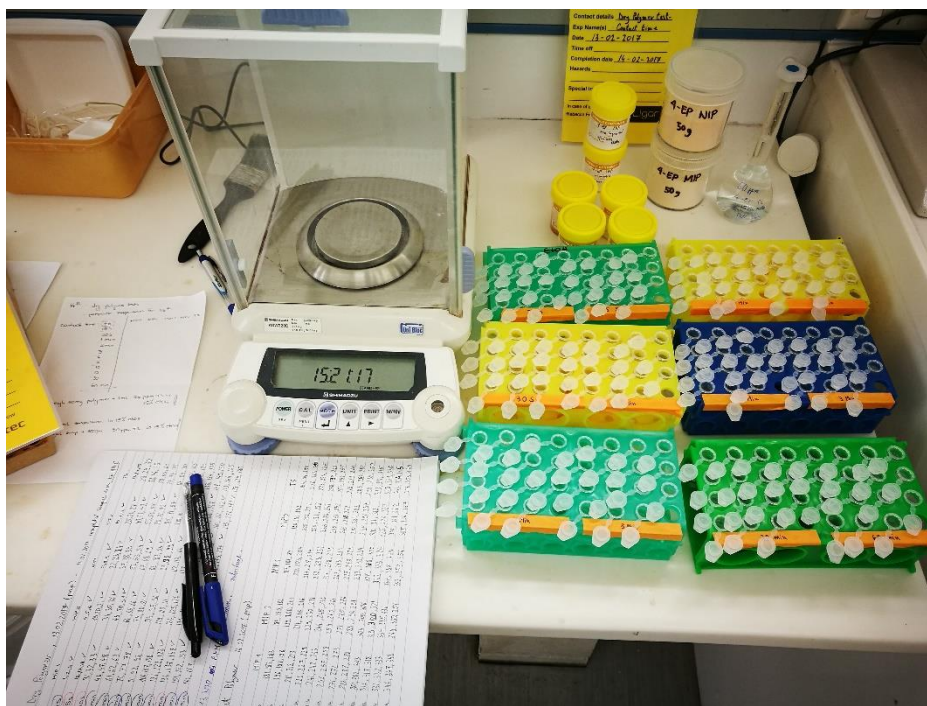
Figure 27. Sample preparation with analytical balance (Shimadzu™ AUW220D)
