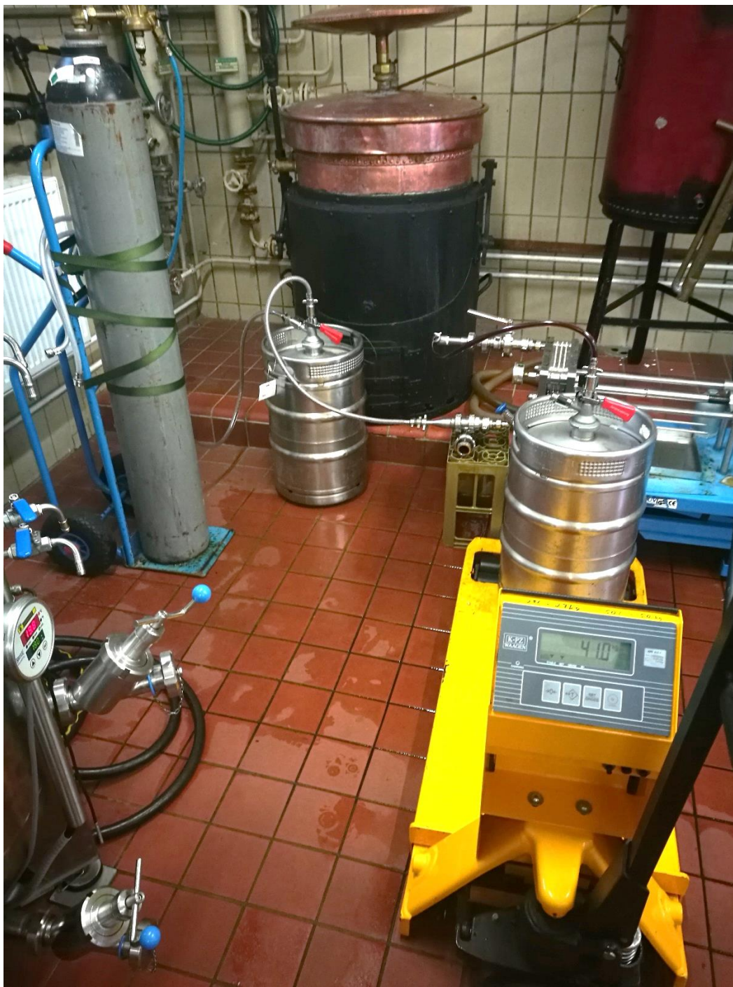
Figure 30. Filtration setup for wine treated with activated carbon beforehand. The wine to be filtered is stored in a stainless-steel keg, and the overpressure from a nitrogen gas tank is used to enable the filtration through Seitz™ EK filter sheets into a new, clean stainless-steel keg
