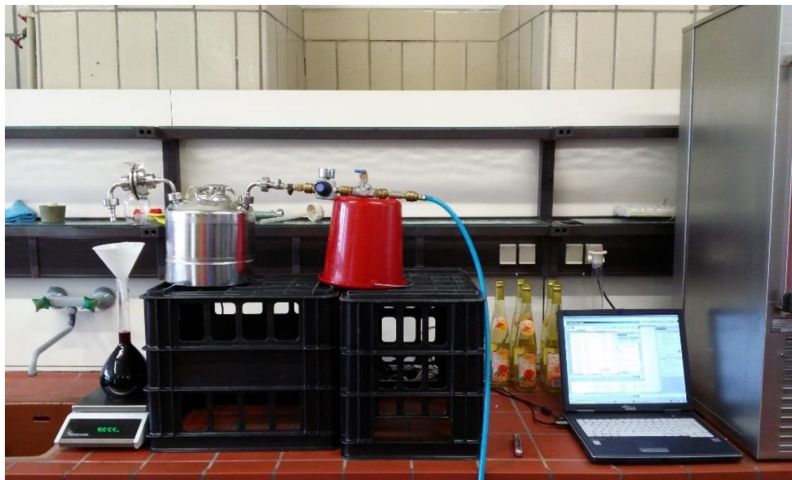
Figure 25. Treatment setup for polymer-embedded filter sheets
