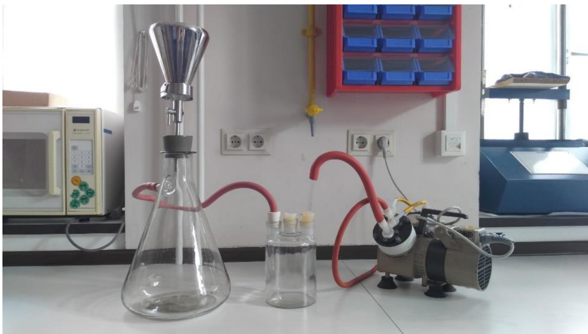
Figure 26. Treatment setup for polymer powder pre-coated on a membrane
