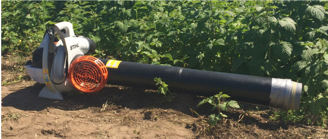
Figure 21: G-Vac suction sampler (modified Stihl SH 56).
