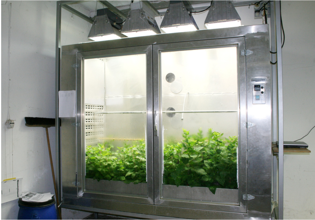
Figure 28: Heating cabinet used in the heat therapy experiment with blackberry plants currently inside. (Figure courtesy of Dr. Christa Lankes)
