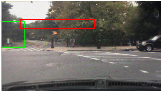
Figure 4: Image from BDD100k with added noise and degraded by an optical model, with ROIs from figures 5 (red) and 6 (green)
