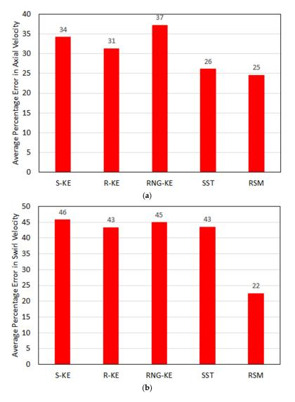
**Figure 9.** Average percentage errors in (**a**) axial and (**b**) swirl velocity predictions for all considered turbulence models.
