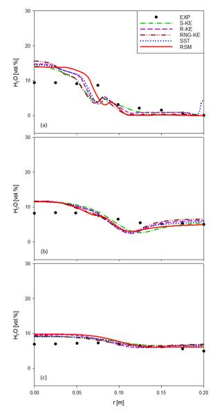
**Figure 11.** Measured [30] and predicted radial profiles of  $H_2O$  volume fractions at three axial stations: (a) x/D = 1.0, (b) x/D = 3.0, (c) x/D = 6.0.
