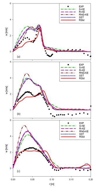
**Figure 8.** Measured [61] and predicted radial profiles of swirl velocity (w) at three axial stations: (a) x/D = 0.5, (b) x/D = 1.0, (c) x/D = 1.5.
