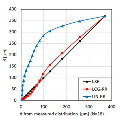
**Figure 15.** Comparison of size class diameters resulting from linear (LIN-RR) and logarithmic (LOG-RR) discretization of the diameter space in RR in comparison with the experimental values (EXP).
