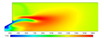
**Figure 6.** Predicted temperature (K) distribution by RSM in burner nearfield for  $x \le 600$  mm.
