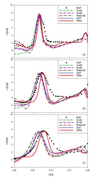
**Figure 7.** Measured [61] and predicted radial profiles of axial velocity (u) at three axial stations: (a) u at x/D = 0.5, (b) u at x/D = 1.0, (c) u at x/D = 1.5.
