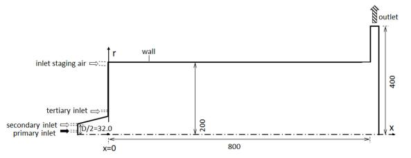
Figure 2. Solution domain, boundaries (drawn not to scale, dimension in mm).
