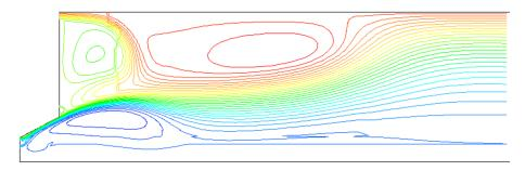
**Figure 4.** Predicted streamline pattern by the RSM in burner nearfield, for  $x \le 600$  mm.
