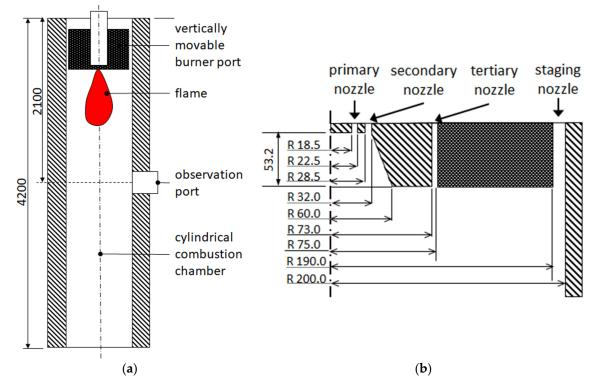
Figure 1. Depiction of test rig from RWTH Aachen University [61]: (a) combustion chamber and (b) swirl burner.
