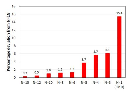
**Figure 18.** Average percentage deviations of centerline temperatures for different N from those of N = 18 (S-KE, M = 30, LOG-RR).
