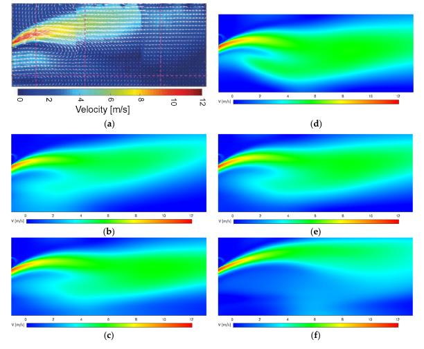
**Figure 5.** Velocity magnitude (m/s) distributions in burner nearfield for  $0 \le x \le 250$  mm and  $0 \le r \le 100$  mm: (a) experiments [61] (b) S-KE, (c) R-KE, (d) RNG-KE, (e) SST, and (f) RSM.
