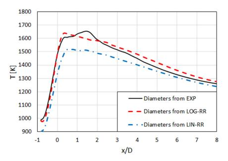
**Figure 16.** Predicted temperature profiles along furnace axis with diameters of size classes obtained from experiments (EXP), logarithmic Rosin–Rammler (LOG-RR), and linear Rosin–Rammler (LIN-RR) distributions (S-KE, N = 18, M = 20).
