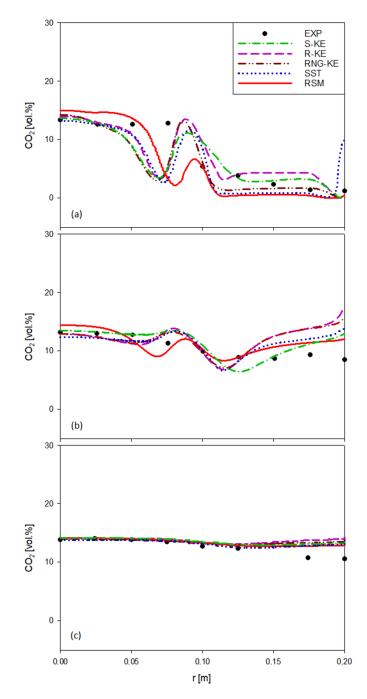
**Figure 10.** Measured [30] and predicted radial profiles of CO<sub>2</sub> volume fractions at three axial stations: (a) x/D = 1.0, (b) x/D = 3.0, (c) x/D = 6.0.
