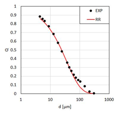
Figure 14. The measured (EXP) and Rosin–Rammler (RR) distributions.
