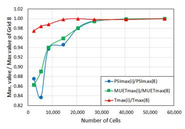
**Figure 3.** Variation of normalized maximum stream function, turbulent viscosity, and temperature predicted by different grids.
