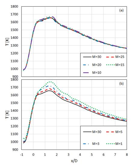
**Figure 12.** Variation of predicted temperature along furnace axis with varying M, (**a**) M = 30, 25, 20, 15, 10, (**b**) M = 30, 5, 3, 1 (S-KE, N = 18).
