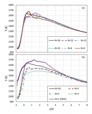
**Figure 17.** Variation of predicted temperature along furnace axis with varying N: (**a**) N = 18, 15, 12, 10, 8, 6, (**b**) N = 18, 5, 4, 3, 1 (S-KE, M = 20, LOG-RR).
