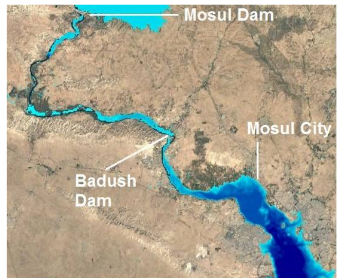
Fig. 1. Predicted flooding after Mosul dam break.
