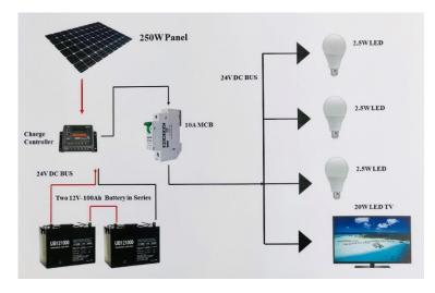
Sunlight is directly changed into electricity by using solar cells. When light hits the solar panels, their photons (particles of sunlight) are converted into electrons of direct current (DC) electricity. The electrons flow out of the solar panel and into an inverter and other electrical safety devices; the energy produced that way is stored in batteries. A net energy meter keeps track of the all the power the solar system produces.
