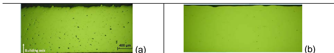
Figure 2. Optical light microscopy image of an SLM processed AISI 316L (a) before re-melting; porosity= 0.77%, density= 99.23% (b) after re-melting; porosity= 0.036%, density= 99.96% [3]. Same scale bars.
