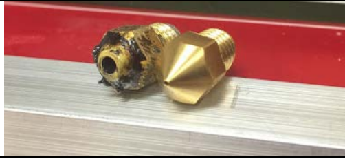
Figure 4. FFF machine brass nozzle showing material abrasive wear after printing of 750 g of carbon fiber reinforced ABS. Starting nozzle size was 1 mm.
