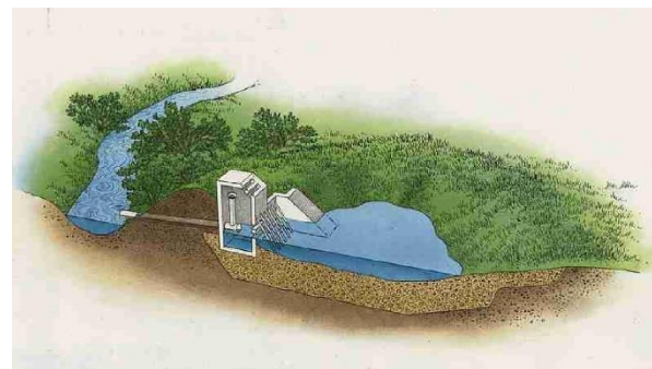
Figure 22 Storage Basin as Components of the nature-oriented handling of rainwater (German Berger und Florian Ettinger 2016)
