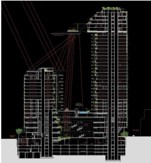
Figure 29 Path of redirected sunlight (Jean Nouvel und Bertram Beissel 2014)
