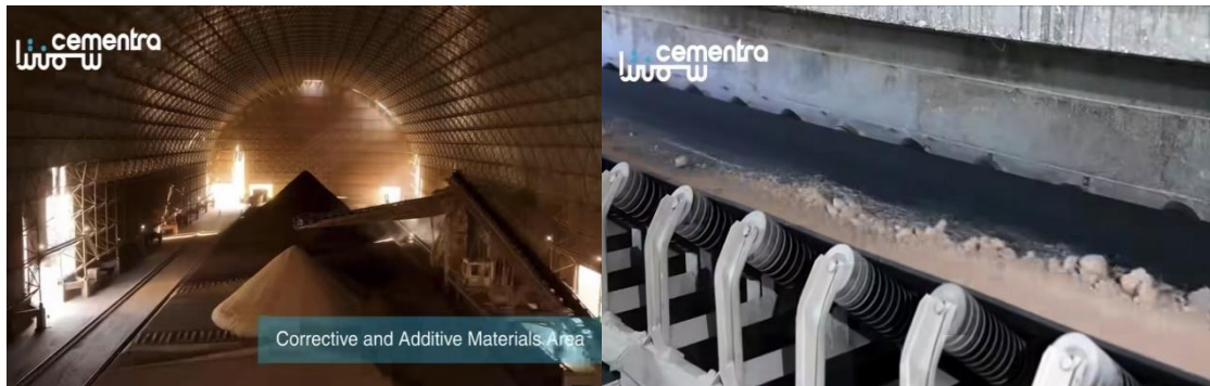
Figure 16, primary metering and proportioning device followed by belt weigh feeders, (cementra jordan, n.d.)
