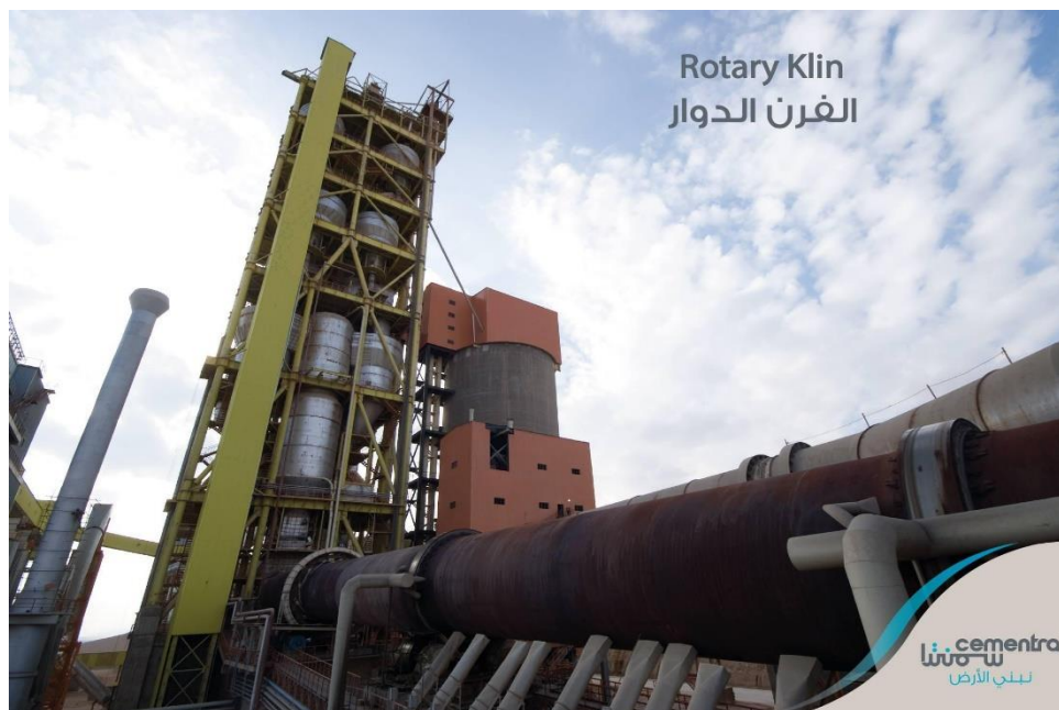
Figure 18, Rotary Kiln, (cementra jordan, n.d.)
