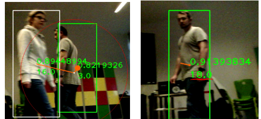
Fig. 5. The robot is able to maintain a stable tracking, even though the TrackID changes from 3 to 18.
