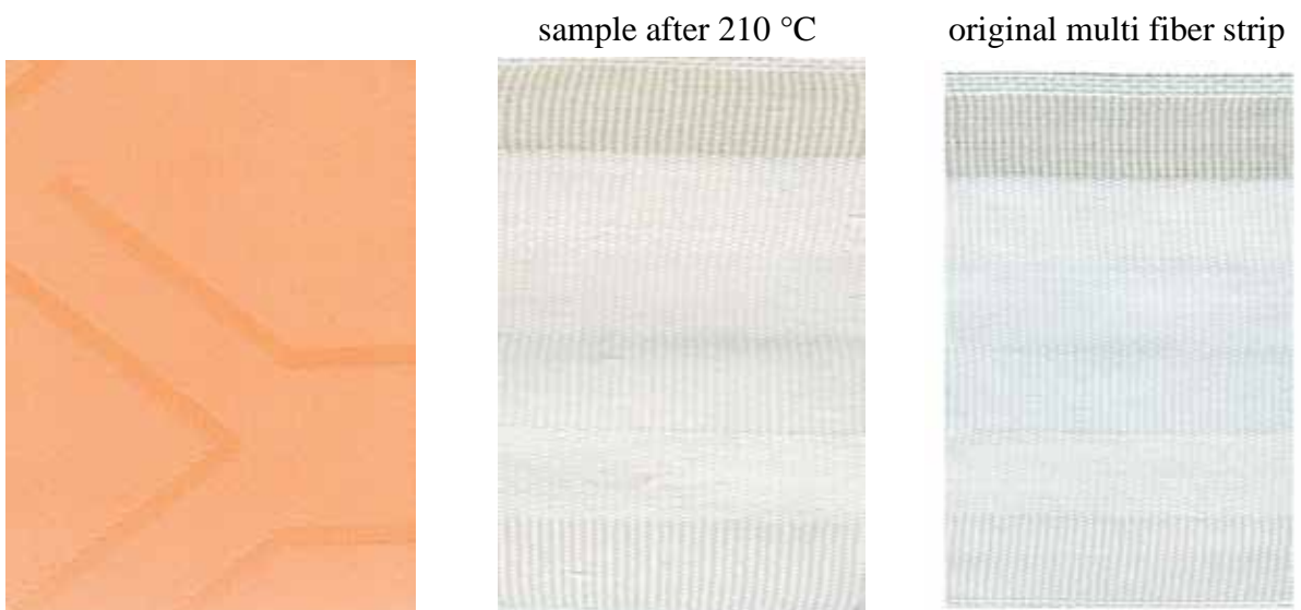
Figure 220: aNIR ® Dianix ® Yellow Brown CC pale shade (Setup 2) sample after 210 °C
