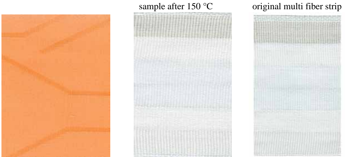
Figure 209: aNIR ® Dianix ® Yellow Brown XF2 pale shade (Setup 2) sample after 150 °C
