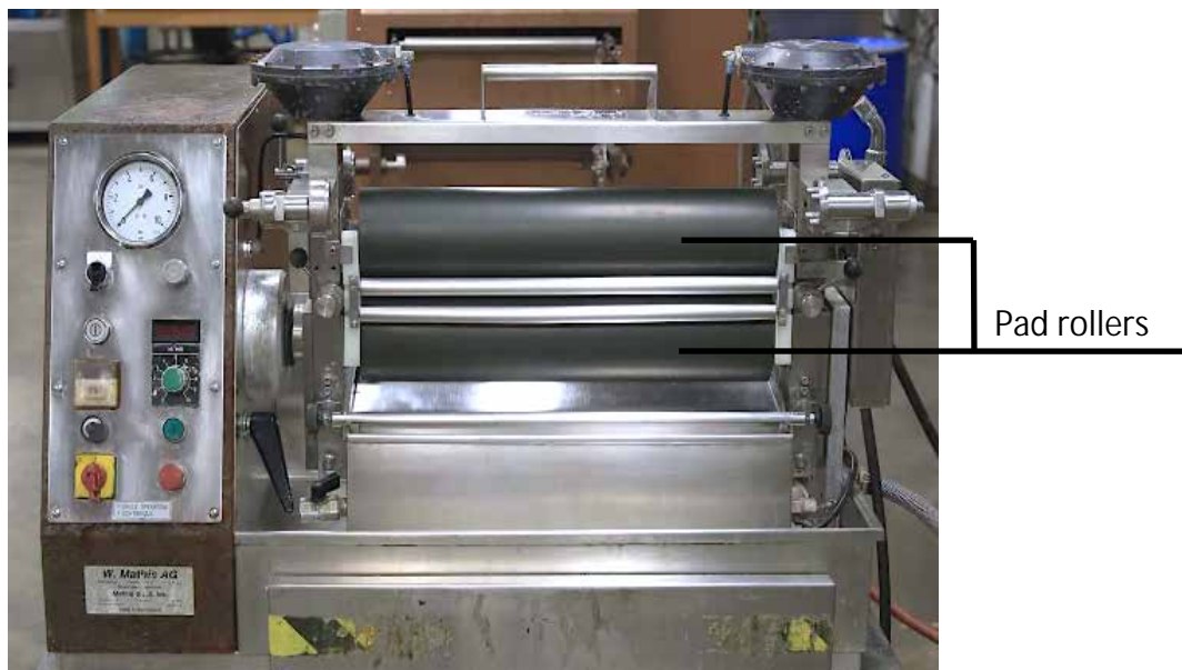
Figure 15: Lab padder (source: own picture)
