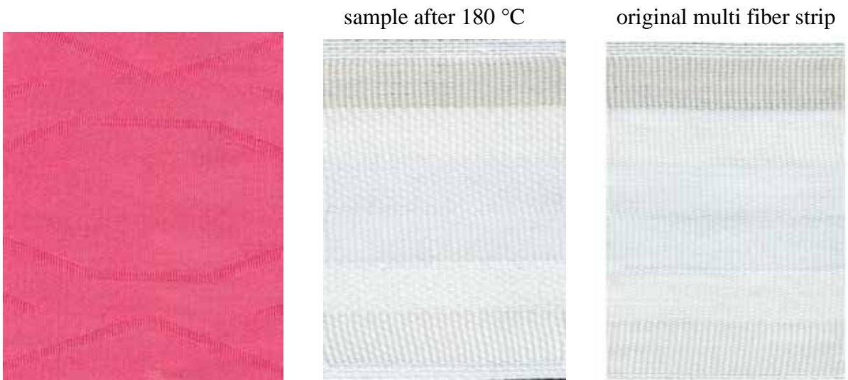
Figure 156: convection process Dianix® Rubine XF2 pale shade sample after 180 °C
