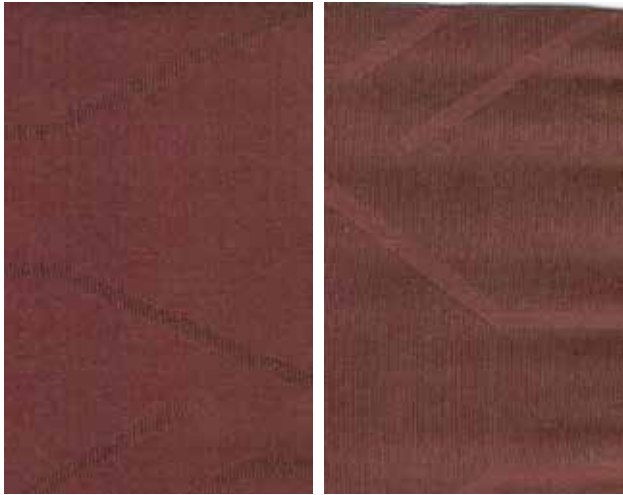
Figure 65: Rotating Atomizer (spray) technology Dianix ® Trichrome CC Brown (Ambient air dried with convection oven thermosoling) (own picture)
