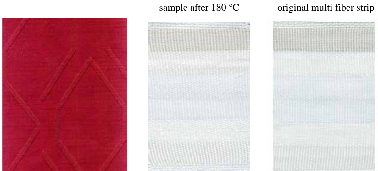
Figure 168: aNIR ® Dianix ® Rubine XF2 medium shade (Setup 1) sample after 180 °C
