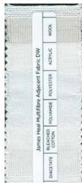
Figure 43: James Heal Multifiber Adjacent fabric DW (own picture)
