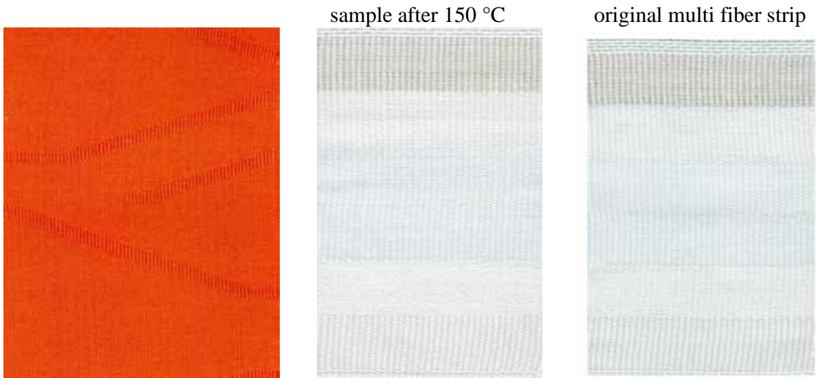
Figure 194: convection process Dianix® Yellow Brown medium shade sample after 150 °C
