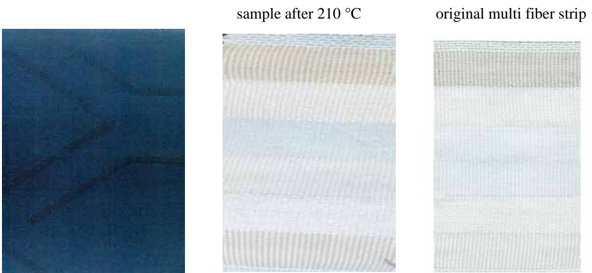
Figure 244: aNIR® Dianix® Navy XF2 dark shade (setup 1) sample after 210 °C
