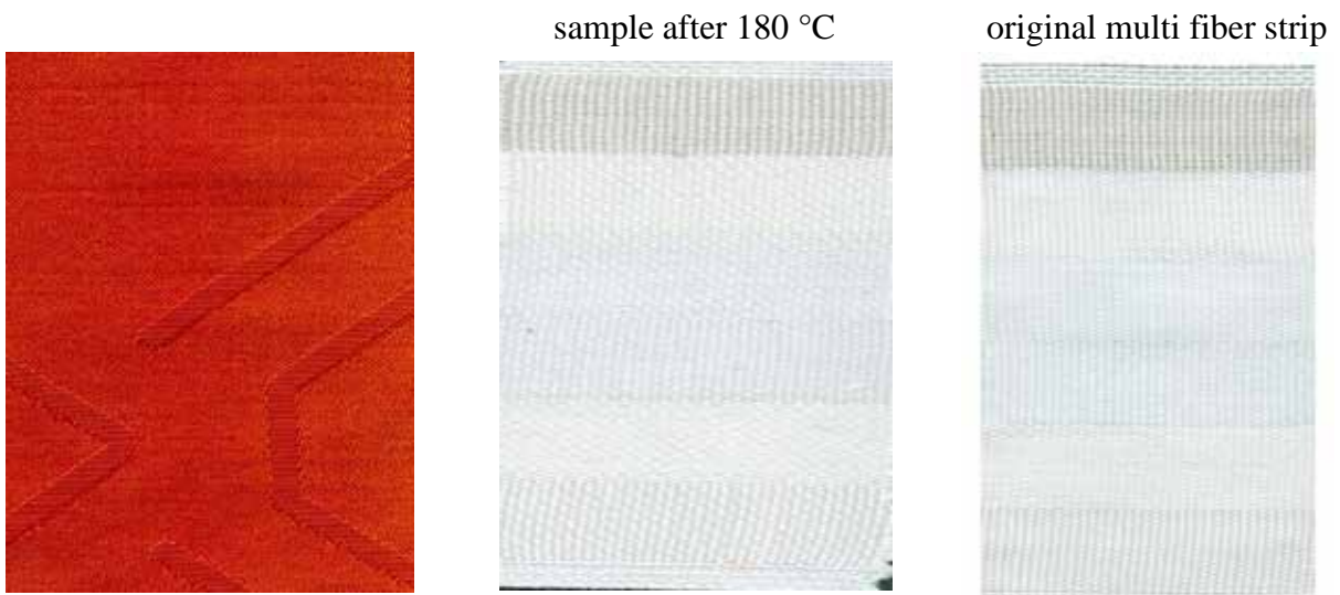
Figure 207: aNIR® Dianix® Yellow Brown XF2 dark shade (Setup 1) sample after 180 °C
