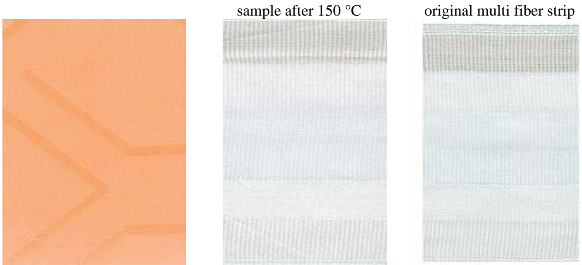
Figure 218: aNIR ® Dianix ® Yellow Brown CC pale shade (Setup 2) sample after 150 °C
