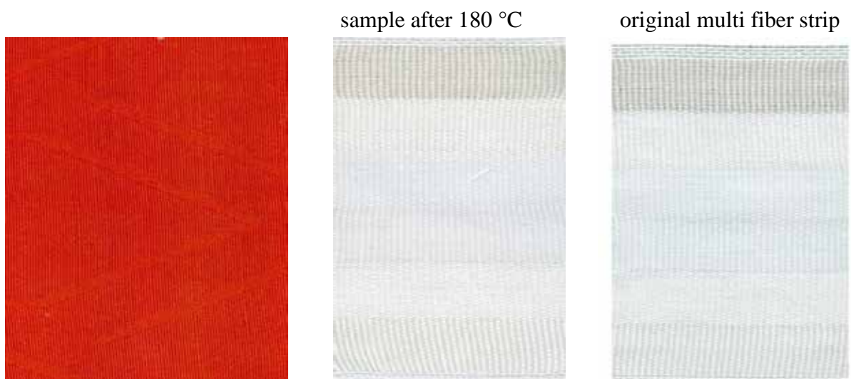
Figure 198: convection process Dianix® Yellow Brown dark shade sample after 180 °C
