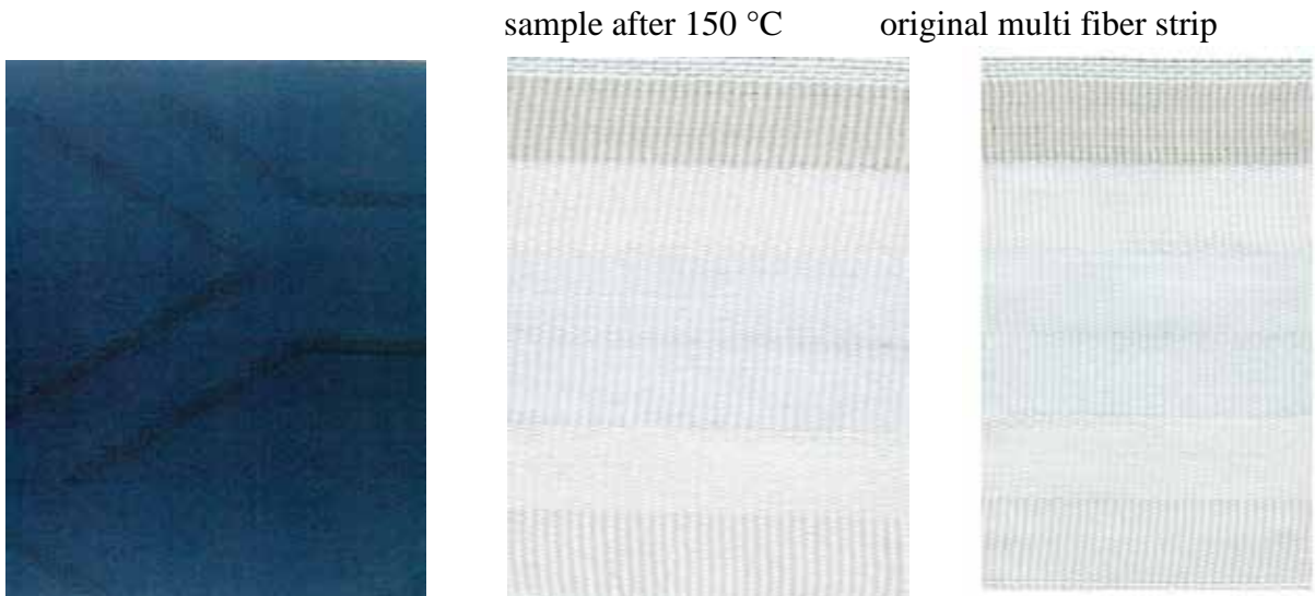
Figure 233: convection process Dianix® Navy XF2 dark shade sample after 150 °C
