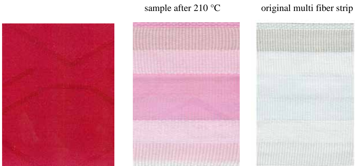
Figure 187: aNIR® Dianix® Rubine CC medium shade (Setup 2) sample after 210 °C
