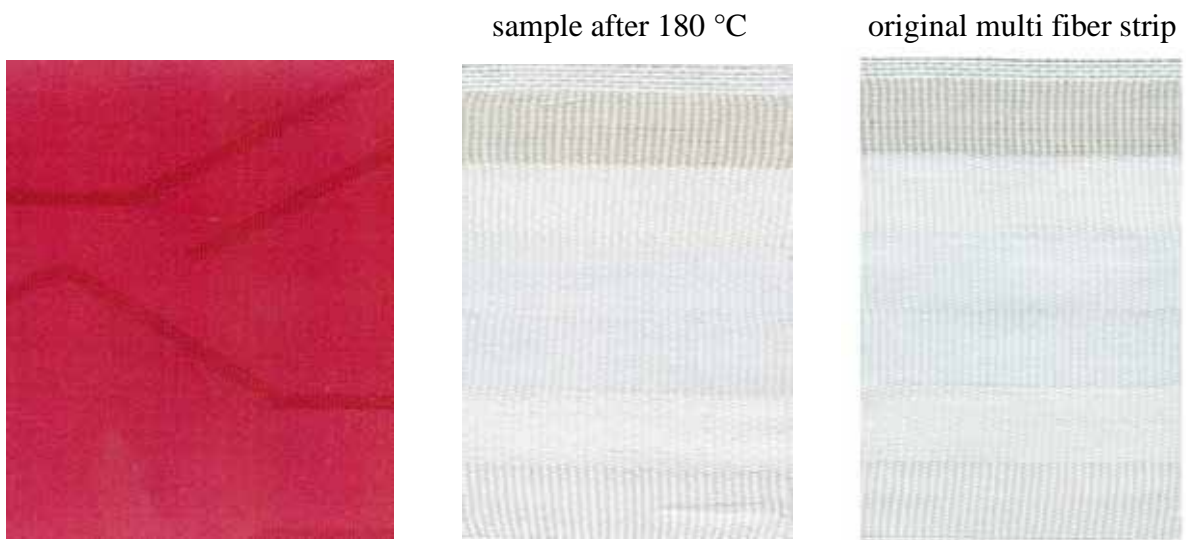
Figure 177: aNIR ® Dianix ® Rubine XF2 medium shade (Setup 2) sample after 180 °C
