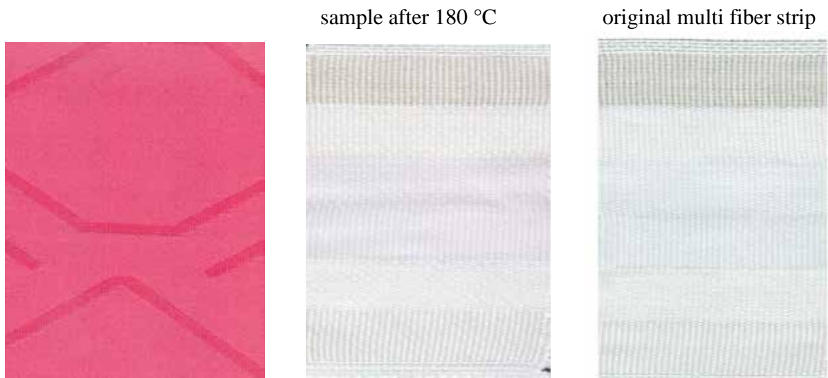
Figure 183: aNIR ® Dianix ® Rubine CC pale shade (Setup 2) sample after 180 °C
