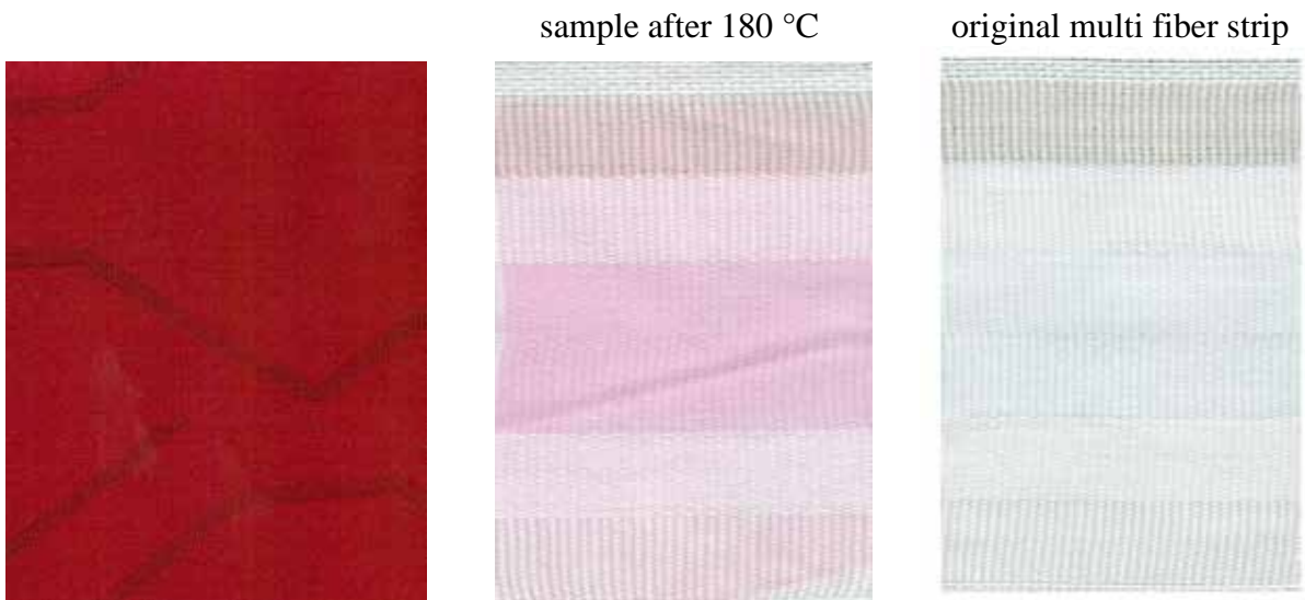
Figure 189: aNIR ® Dianix ® Rubine CC dark shade (Setup 2) sample after 180 °C
