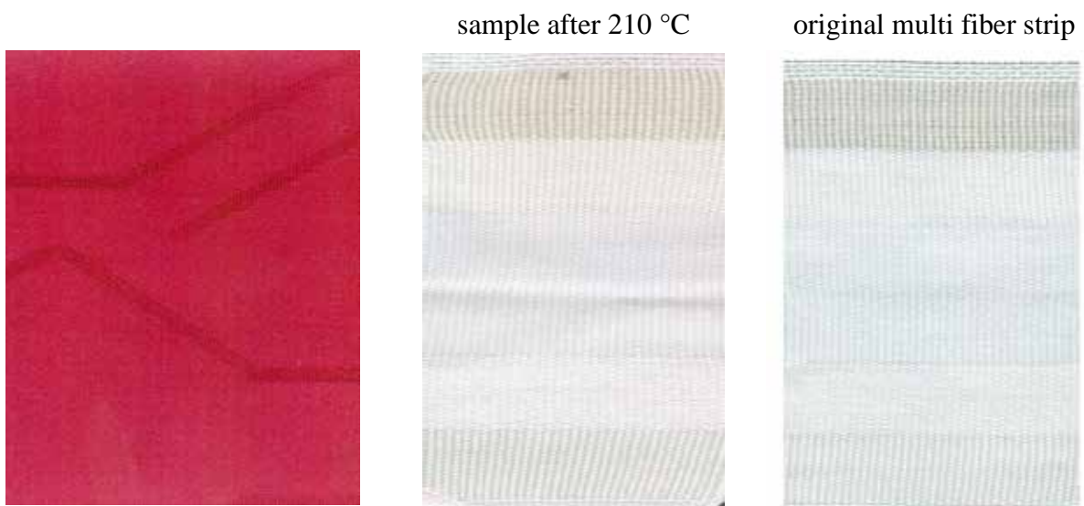
Figure 178: aNIR ® Dianix ® Rubine XF2 medium shade (Setup 2) sample after 210 °C
