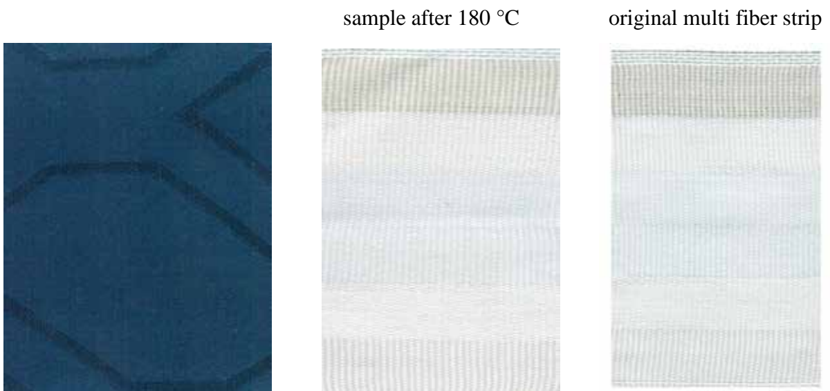
Figure 249: aNIR® Dianix® Navy XF2 medium shade (setup 2) sample after 180 °C
