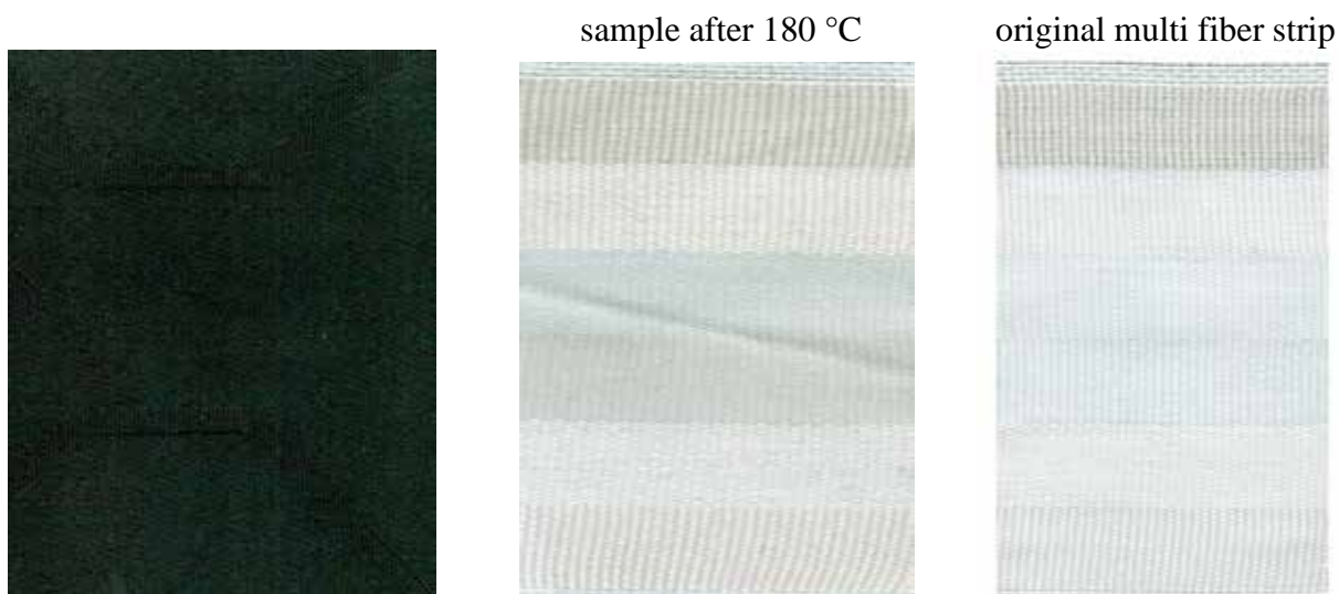
Figure 297: aNIR® Dianix® Black CC-R dark shade (setup 2) sample after 180 °C
