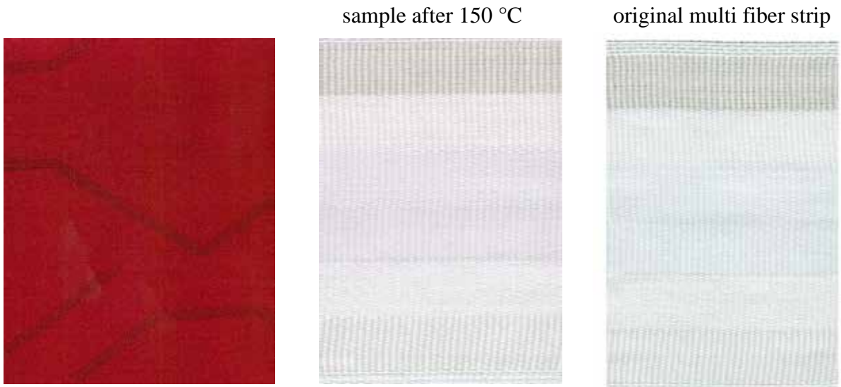
Figure 188: aNIR ® Dianix ® Rubine CC dark shade (Setup 2) sample after 150 °C
