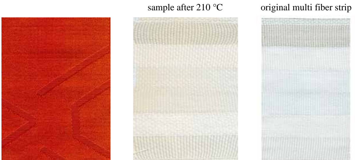
Figure 208: aNIR® Dianix® Yellow Brown XF2 dark shade (Setup 1) sample after 210 °C
