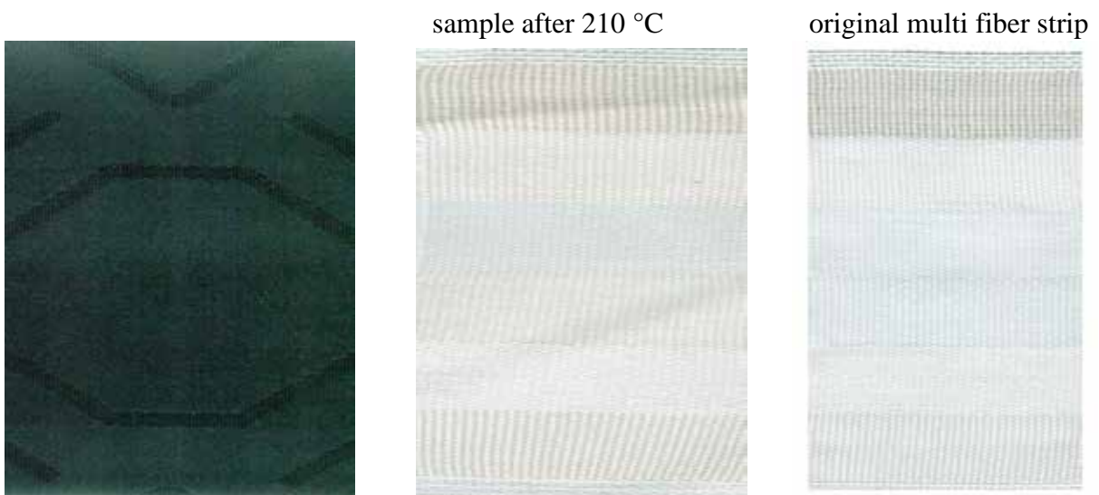
Figure 277: aNIR ® Dianix ® Black XF2 300% medium shade (setup 1) sample after 210 °C
