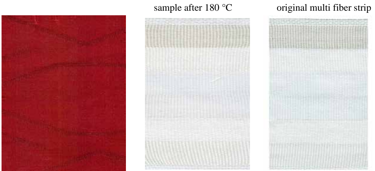
Figure 162: convection process Dianix® Rubine XF2 dark shade sample after 180 °C
