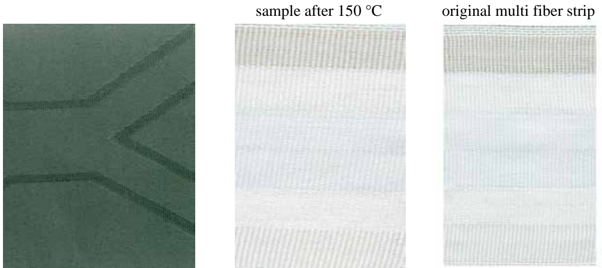
Figure 290: aNIR ® Dianix ® Black CC-R pale shade (setup 2) sample after 150 °C
