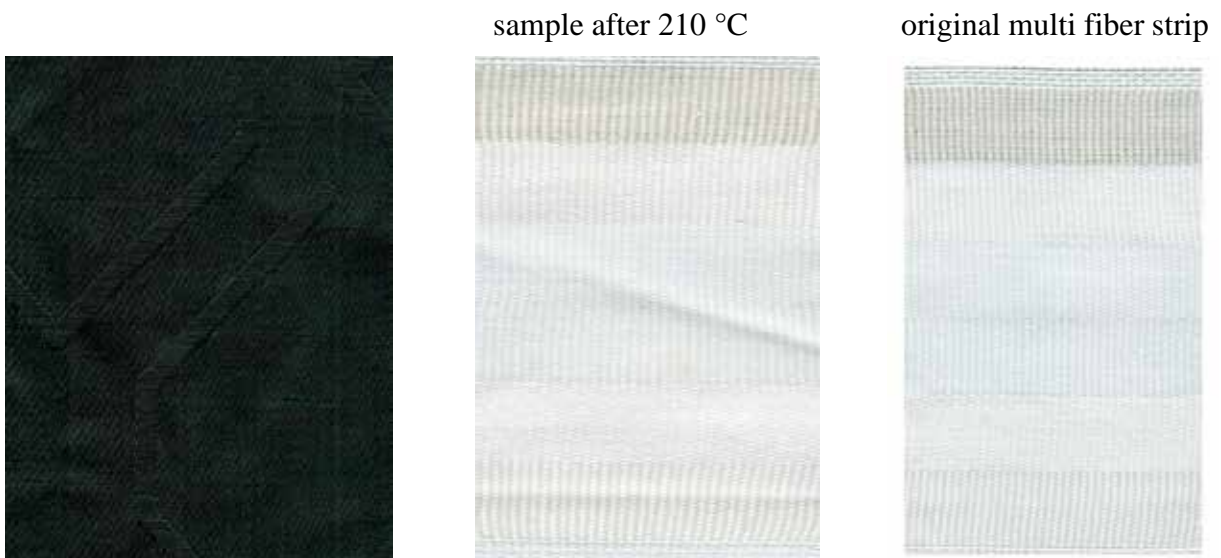
Figure 289: aNIR® Dianix® Black XF2 300% dark shade (setup 2) sample after 210 °C
