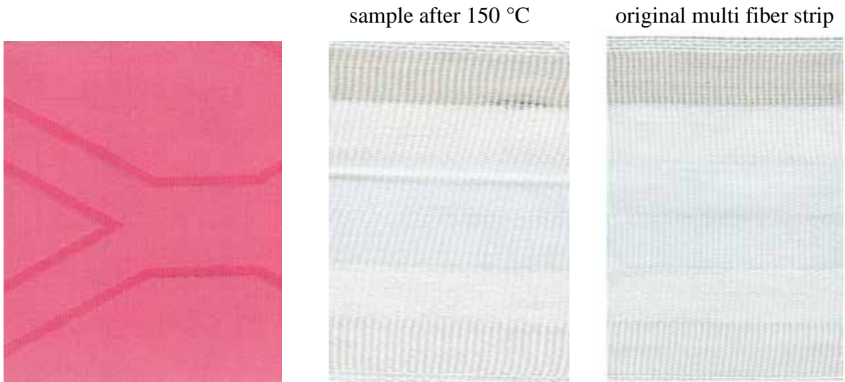
Figure 173: aNIR® Dianix® Rubine XF2 pale shade (Setup 2) sample after 150 °C
