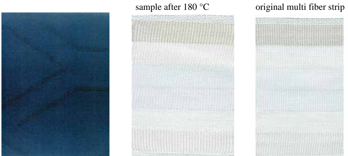
Figure 243: aNIR® Dianix® Navy XF2 dark shade (setup 1) sample after 180 °C
