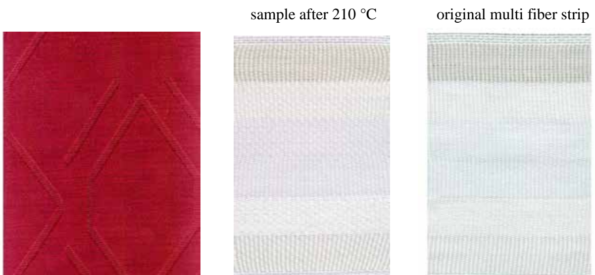
Figure 169: aNIR ® Dianix ® Rubine XF2 medium shade (Setup 1) sample after 210 °C
