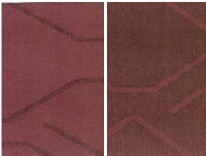
Figure 71: Rotating Atomizer (spray) technology with aNIR® technology process (Dianix® Trichrome CC Brown) setup 2 (own picture)
