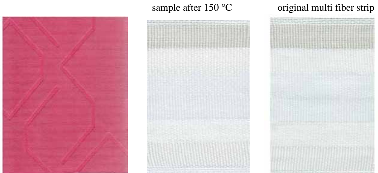
Figure 164: aNIR ® Dianix ® Rubine XF2 pale shade (Setup 1) sample after 150 °C
