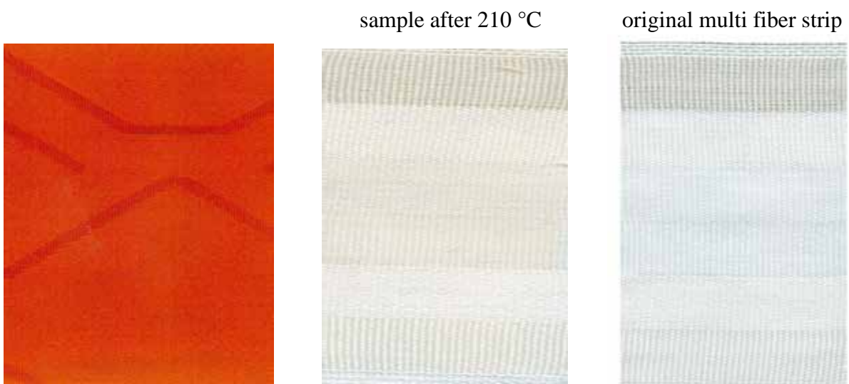
Figure 217: aNIR ® Dianix ® Yellow Brown XF2 dark shade (Setup 2) sample after 210 °C
