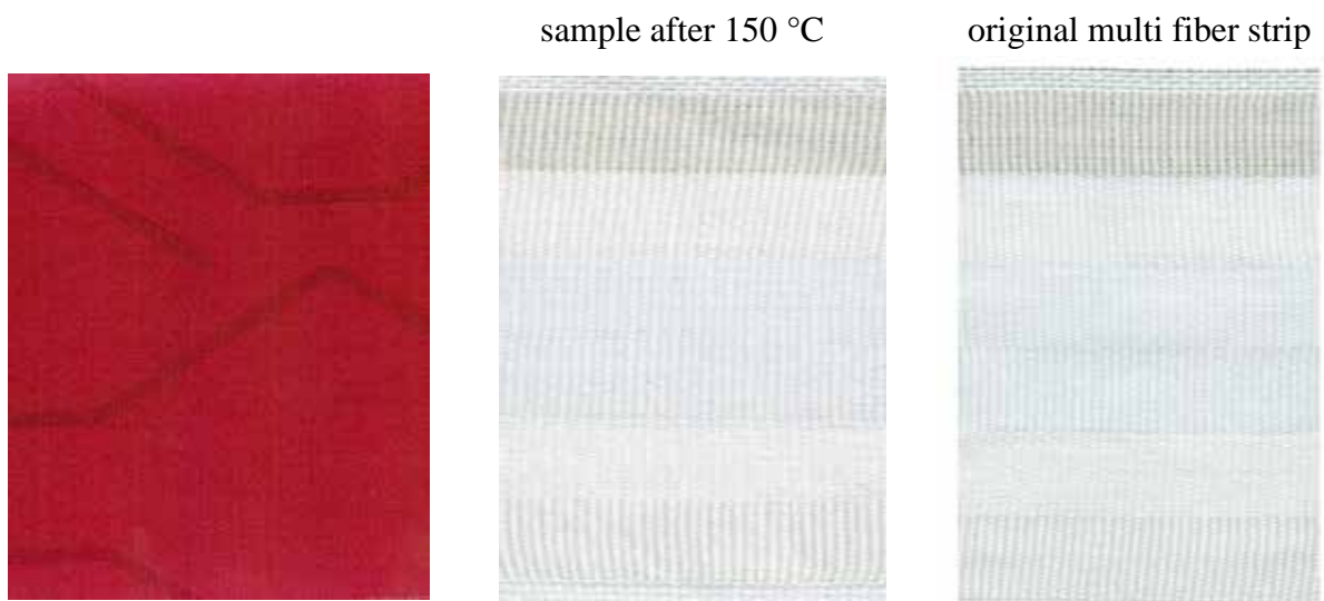
Figure 179: aNIR® Dianix® Rubine XF2 dark shade (Setup 2) sample after 150 °C
