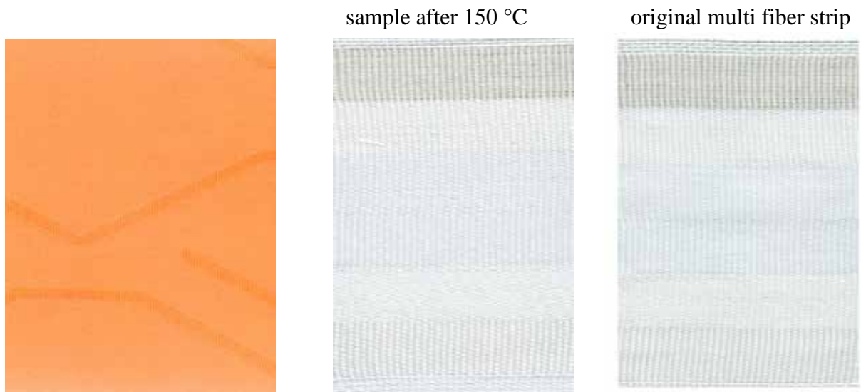
Figure 200: aNIR ® Dianix ® Yellow Brown XF2 pale shade (Setup 1) sample after 150 °C
