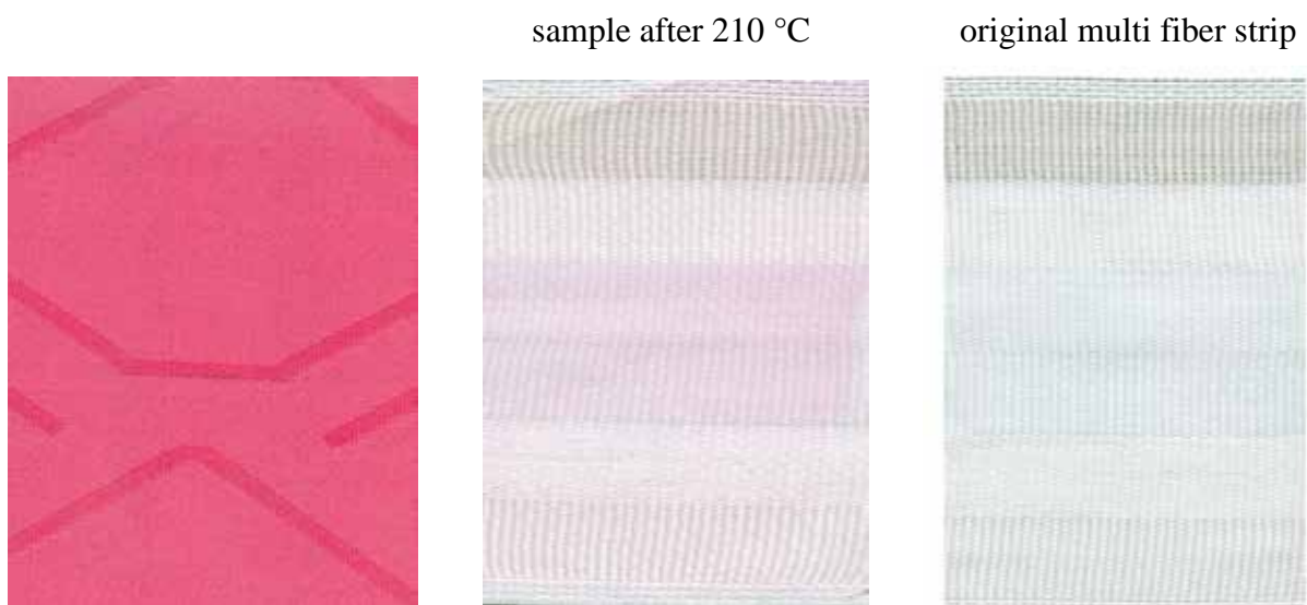
Figure 184: aNIR ® Dianix ® Rubine CC pale shade (Setup 2) sample after 210 °C
