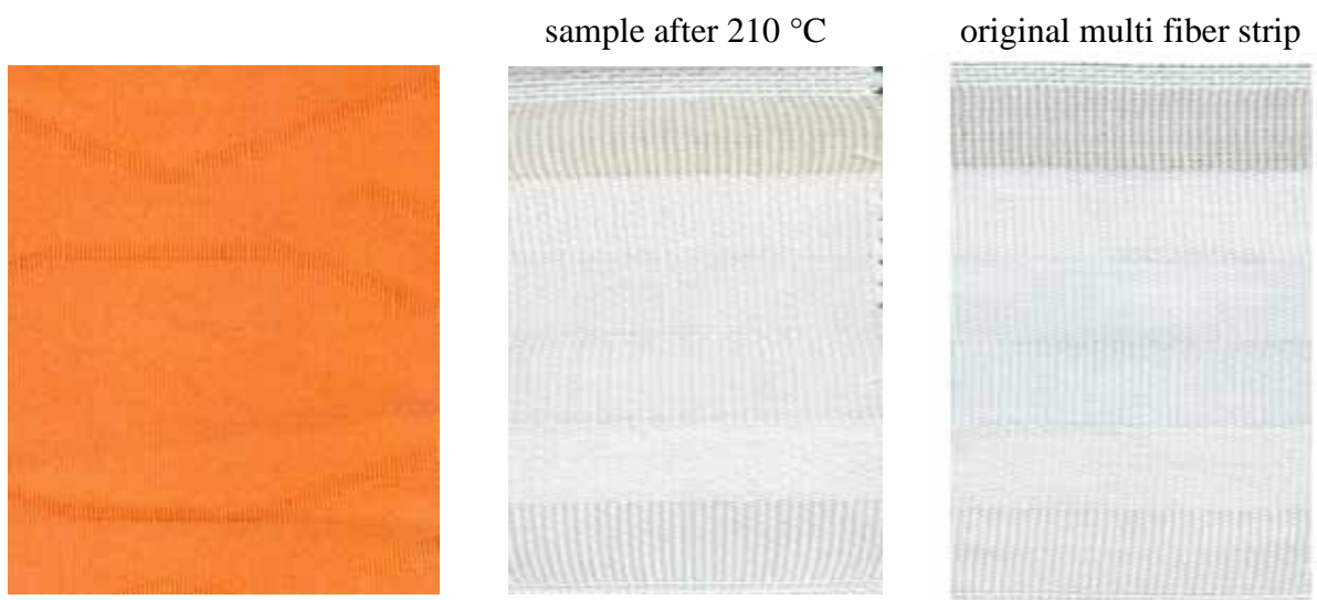
Figure 193: convection process Dianix® Yellow Brown pale shade sample after 210 °C
