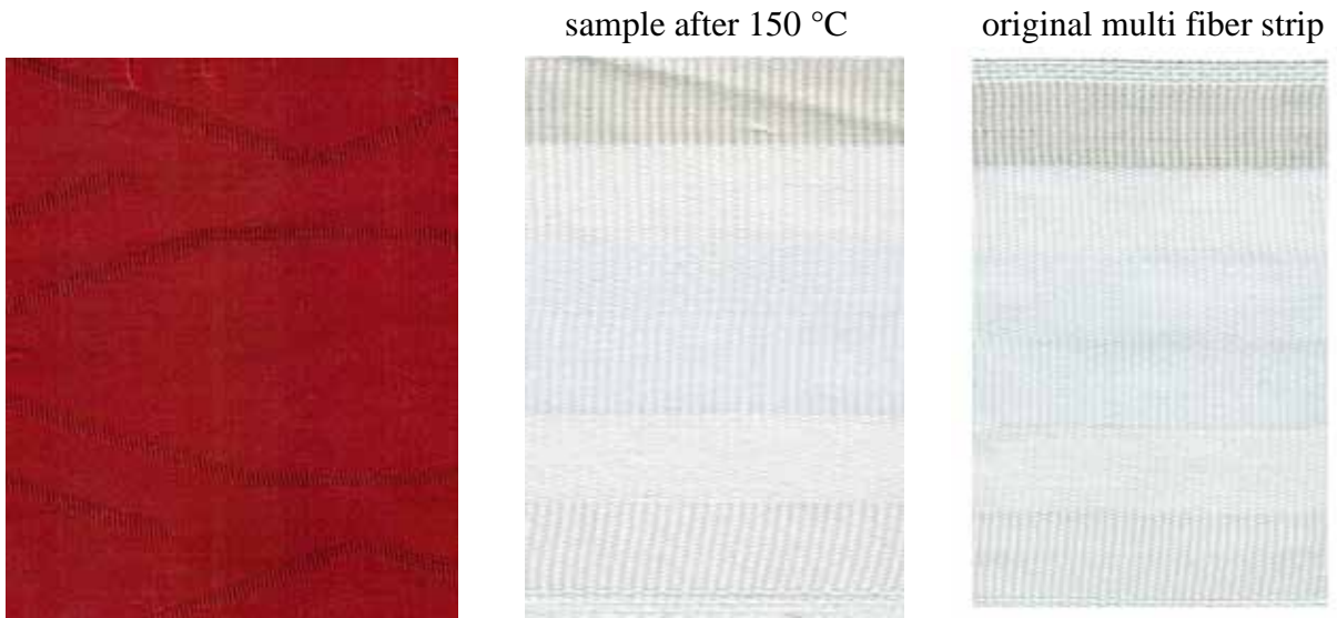
Figure 161: convection process Dianix® Rubine XF2 dark shade sample after 150 °C
