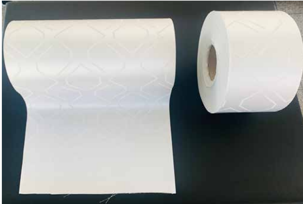
Figure 34: Polyester fiber: Conventional process;left aNIR ® Technology process; right (own picture)
