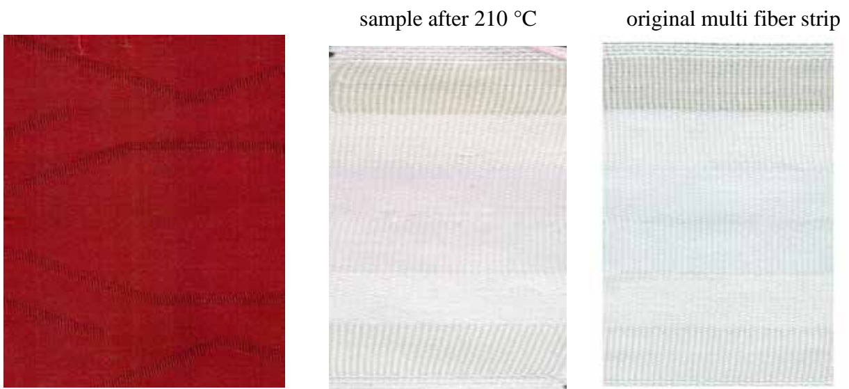
Figure 163: convection process Dianix® Rubine XF2 dark shade sample after 210 °C
