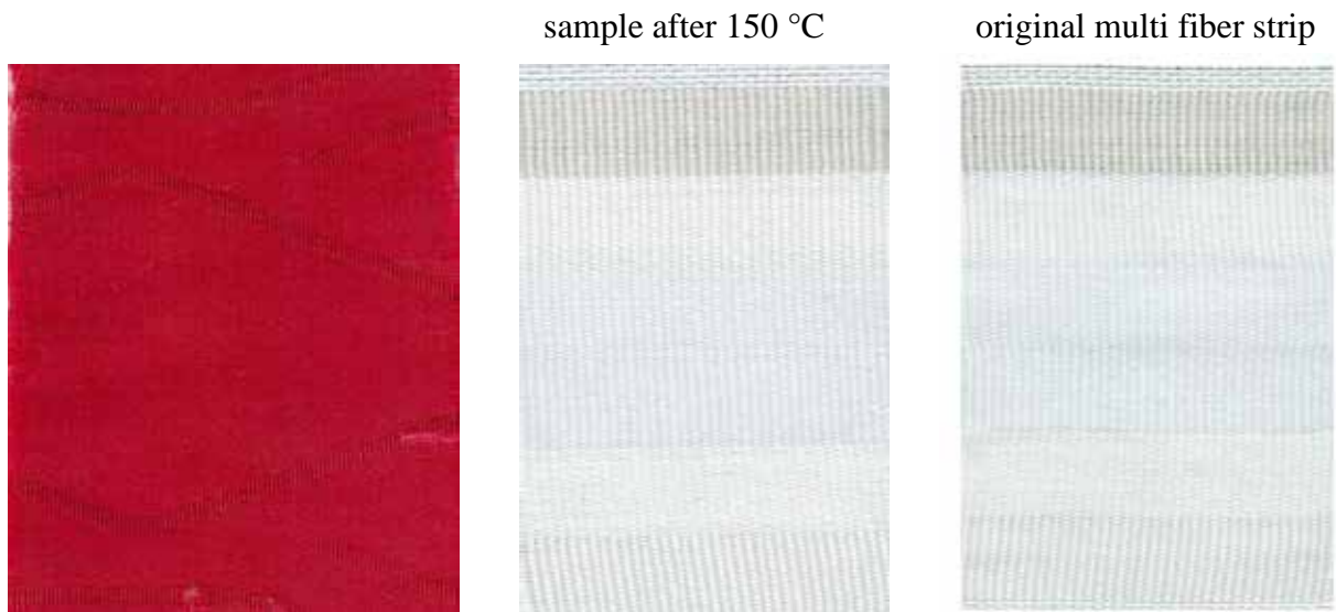
Figure 158: convection process Dianix® Rubine medium shade sample after 150 °C
