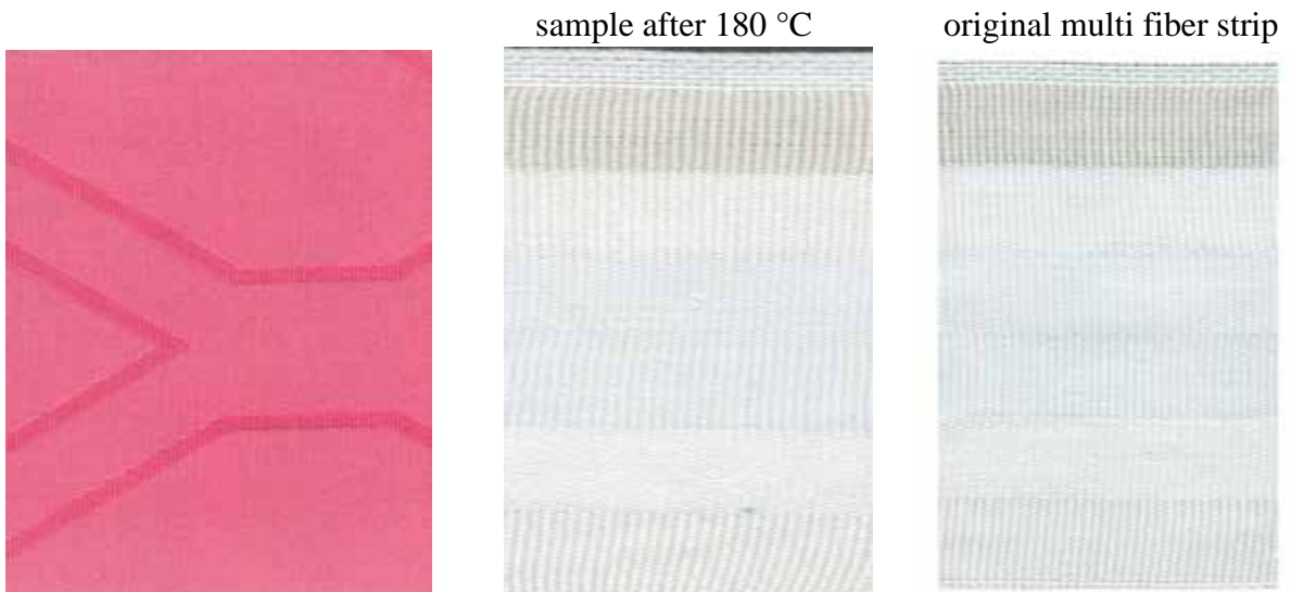
Figure 174: aNIR® Dianix® Rubine XF2 pale shade (Setup 2) sample after 180 °C
