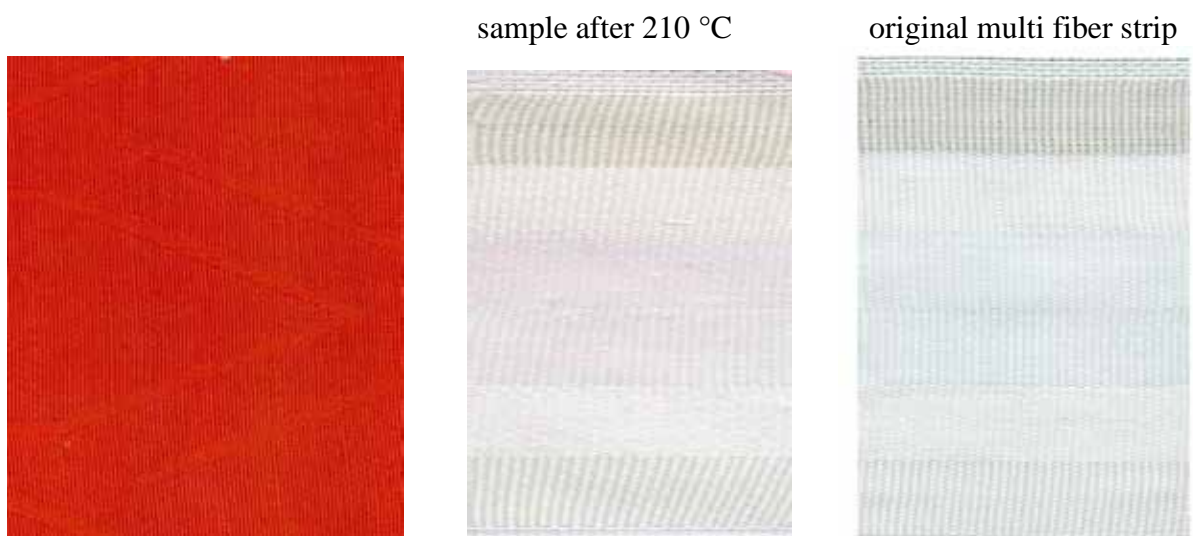
Figure 199: convection process Dianix® Yellow Brown dark shade sample after 210 °C
