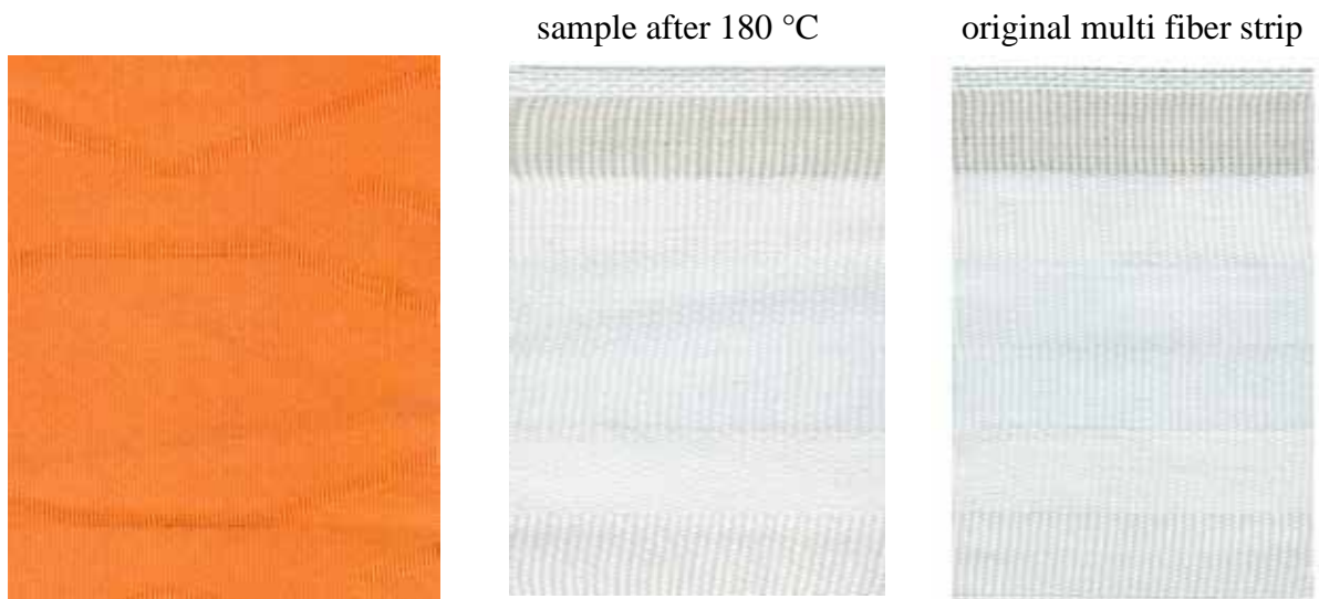
Figure 192: convection process Dianix® Yellow Brown pale shade sample after 180 °C
