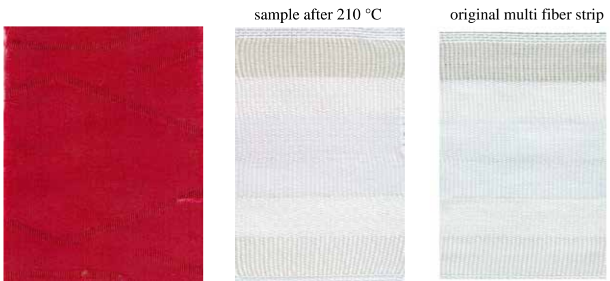
Figure 160: convection process Dianix® Rubine medium shade sample after 210 °C
