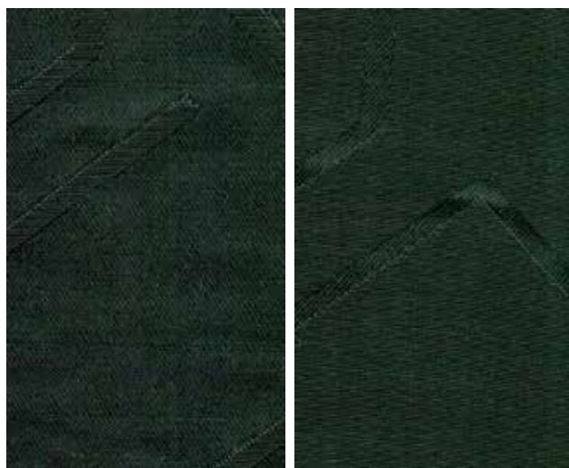
Figure 56: Convection process 30 g/l Dianix® Black CC-R 7 g/l Sera® Gal M-SPR (own picture)
