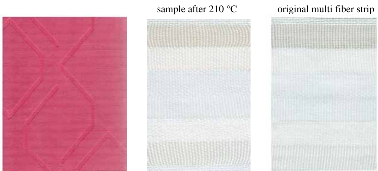
Figure 166: aNIR ™ Dianix ™ Rubine XF2 pale shade (Setup 1) sample after 210 °C
