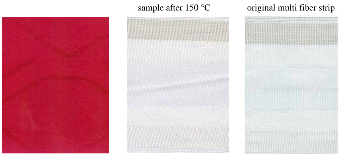
Figure 185: aNIR® Dianix® Rubine CC medium shade (Setup 2) sample after 150 °C
