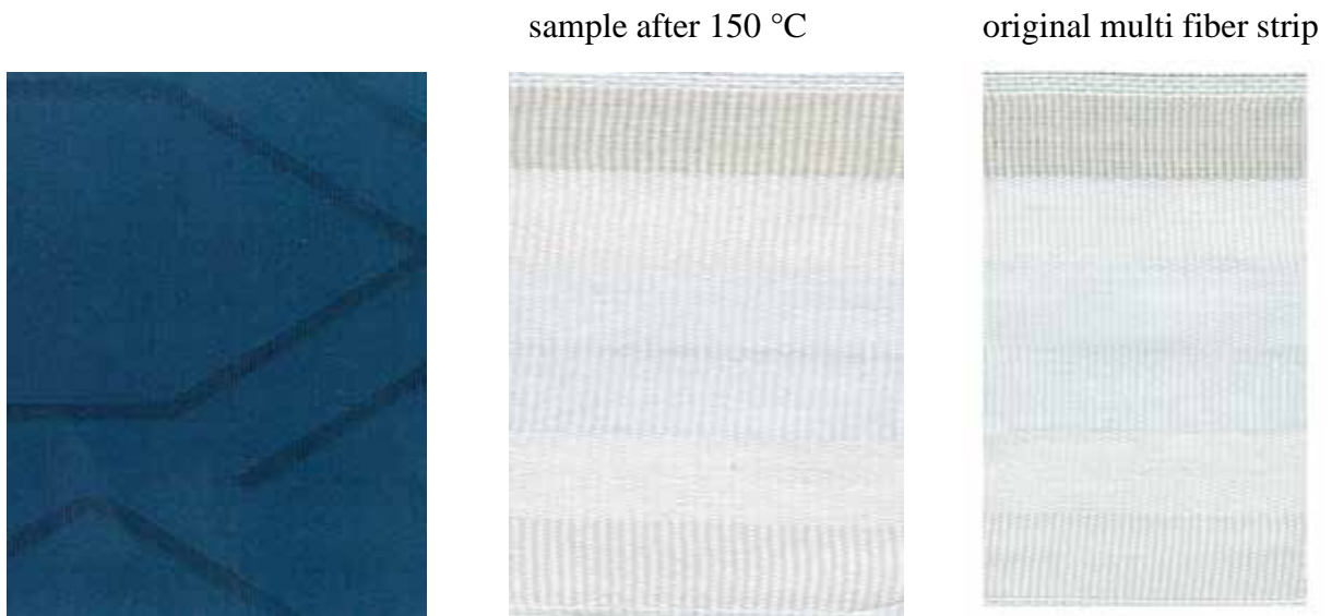
Figure 257: aNIR® Dianix® Navy CC medium shade (setup 2) sample after 150 °C
