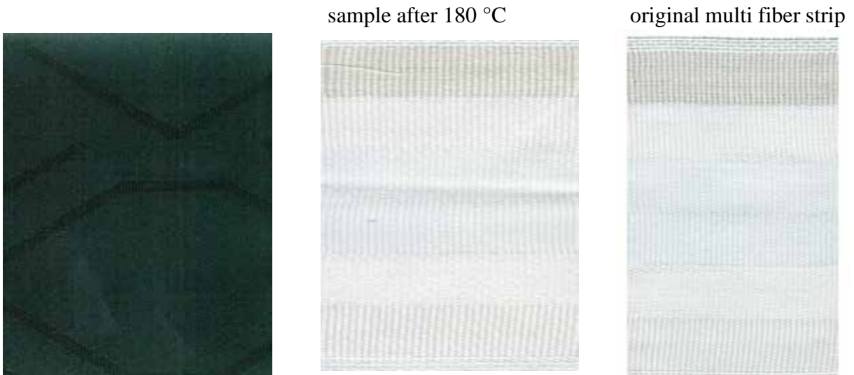
Figure 285: aNIR® Dianix® Black XF2 300% medium shade (setup 2) sample after 180 °C
