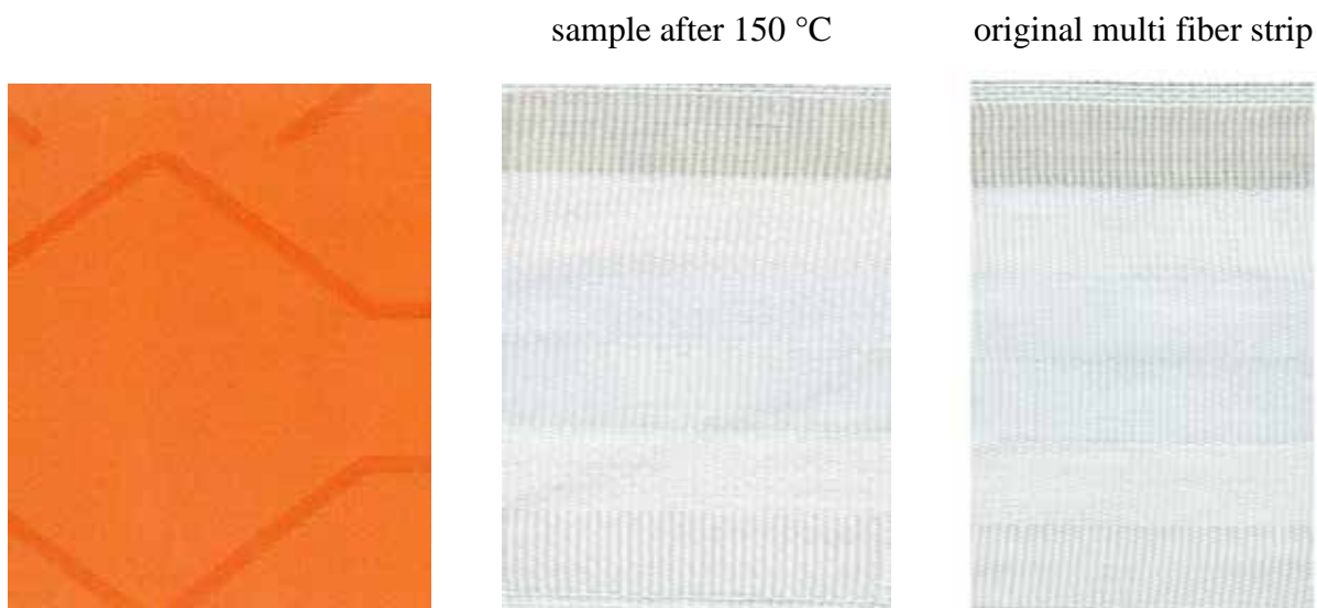
Figure 221: aNIR® Dianix® Yellow Brown CC medium shade (Setup 2) sample after 150 °C
