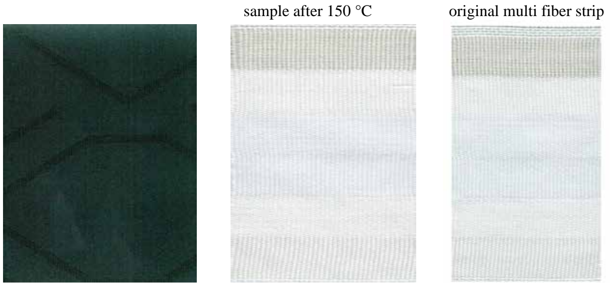
Figure 284: aNIR® Dianix® Black XF2 300% medium shade (setup 2) sample after 150 °C
