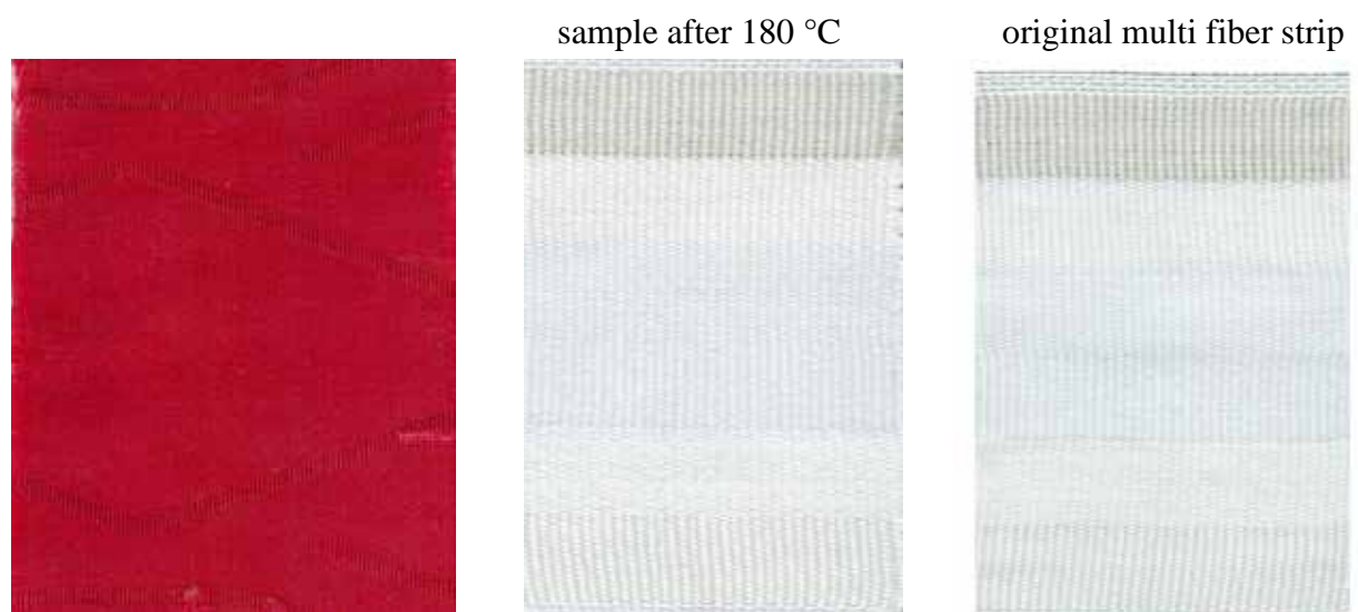
Figure 159: convection process Dianix® Rubine medium shade sample after 180 °C
