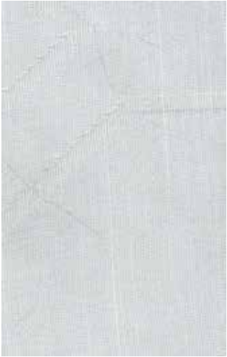
Figure 47: Blank sample (without dye) Thermofixed 215 °C
