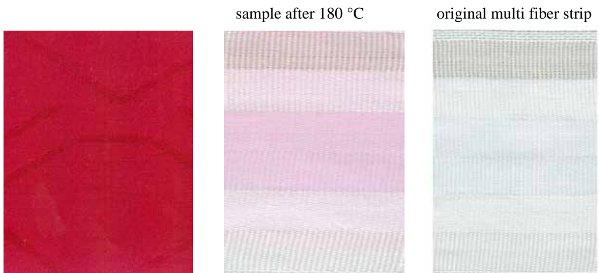
Figure 186: aNIR® Dianix® Rubine CC medium shade (Setup 2) sample after 180 °C
