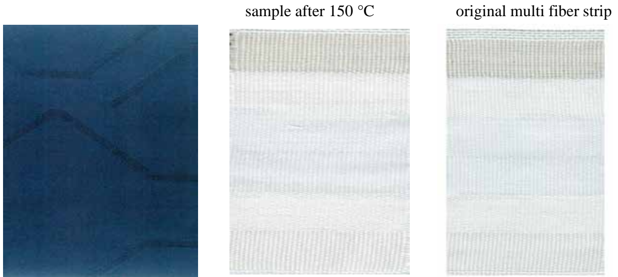
Figure 239: aNIR® Dianix® Navy XF2 medium shade (setup 1) sample after 150 °C
