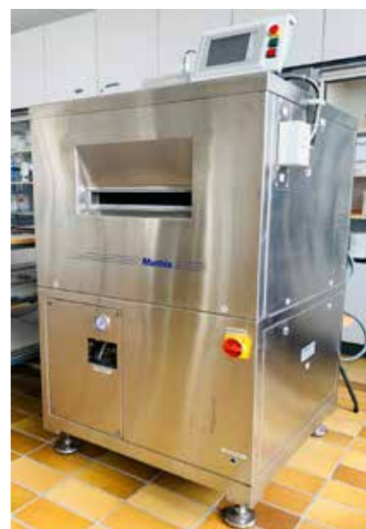
Figure 36: Image of foulard and convection oven dryer and thermosoling unit. (Own picture)
