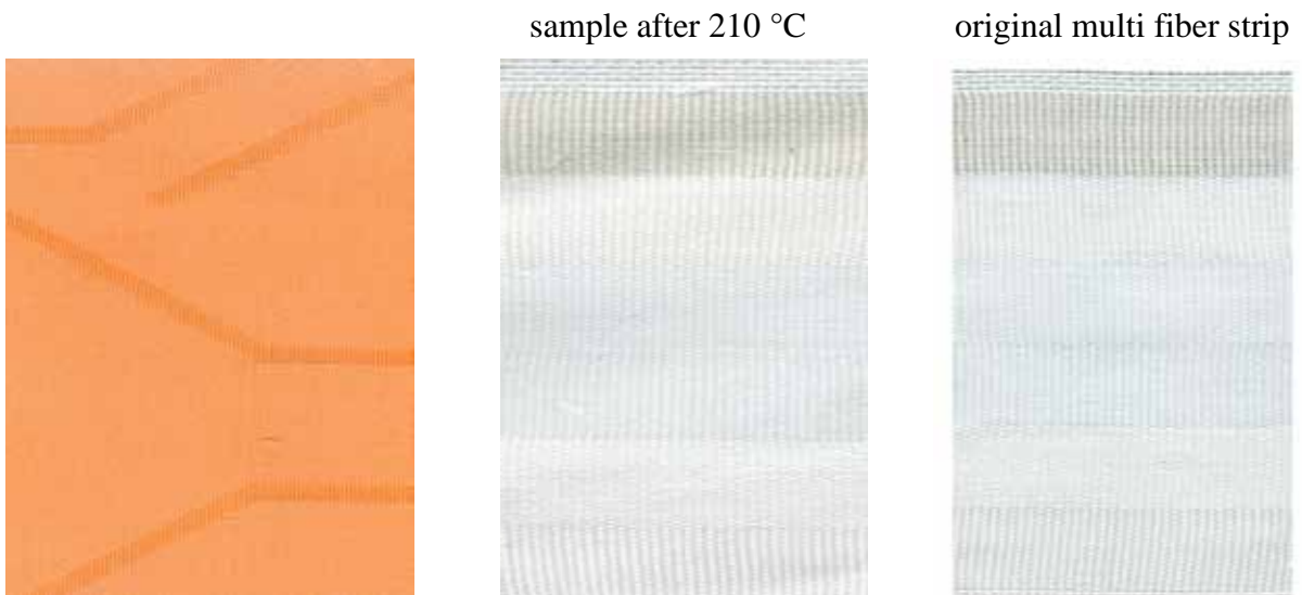
Figure 211: aNIR ® Dianix ® Yellow Brown XF2 pale shade (Setup 2) sample after 210 °C
