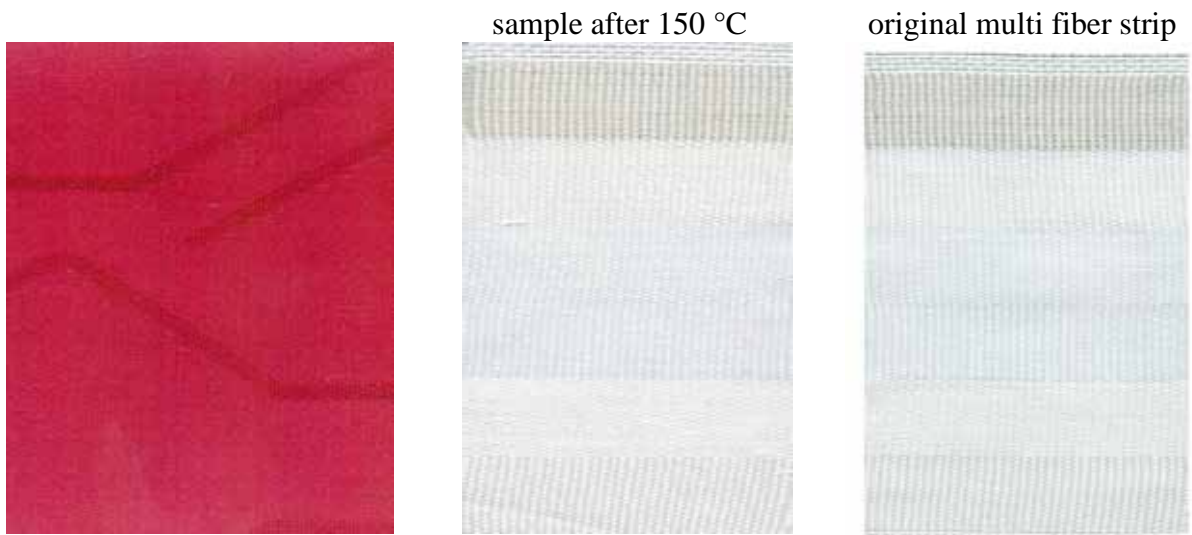
Figure 176: aNIR ® Dianix ® Rubine XF2 medium shade (Setup 2) sample after 150 °C
