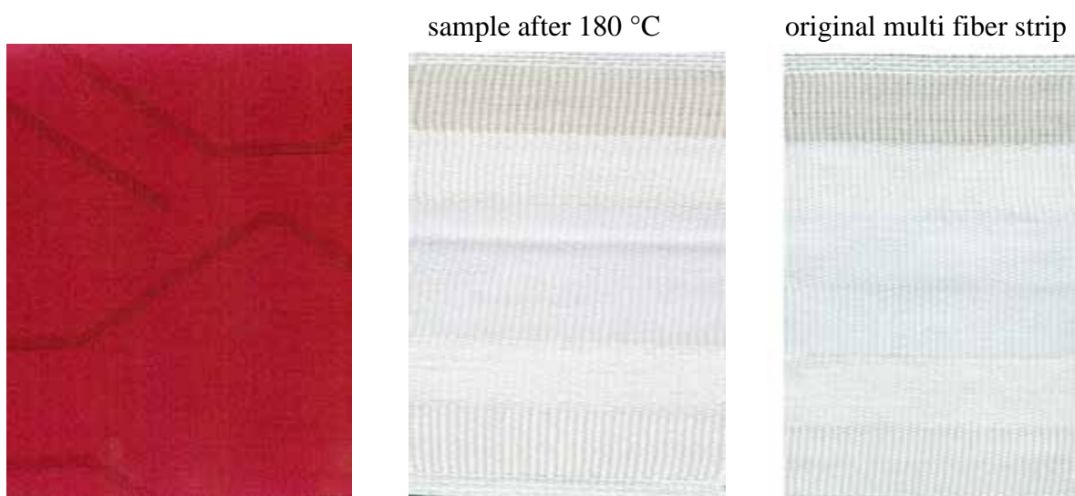
Figure 180: aNIR® Dianix® Rubine XF2 dark shade (Setup 2) sample after 180 °C
