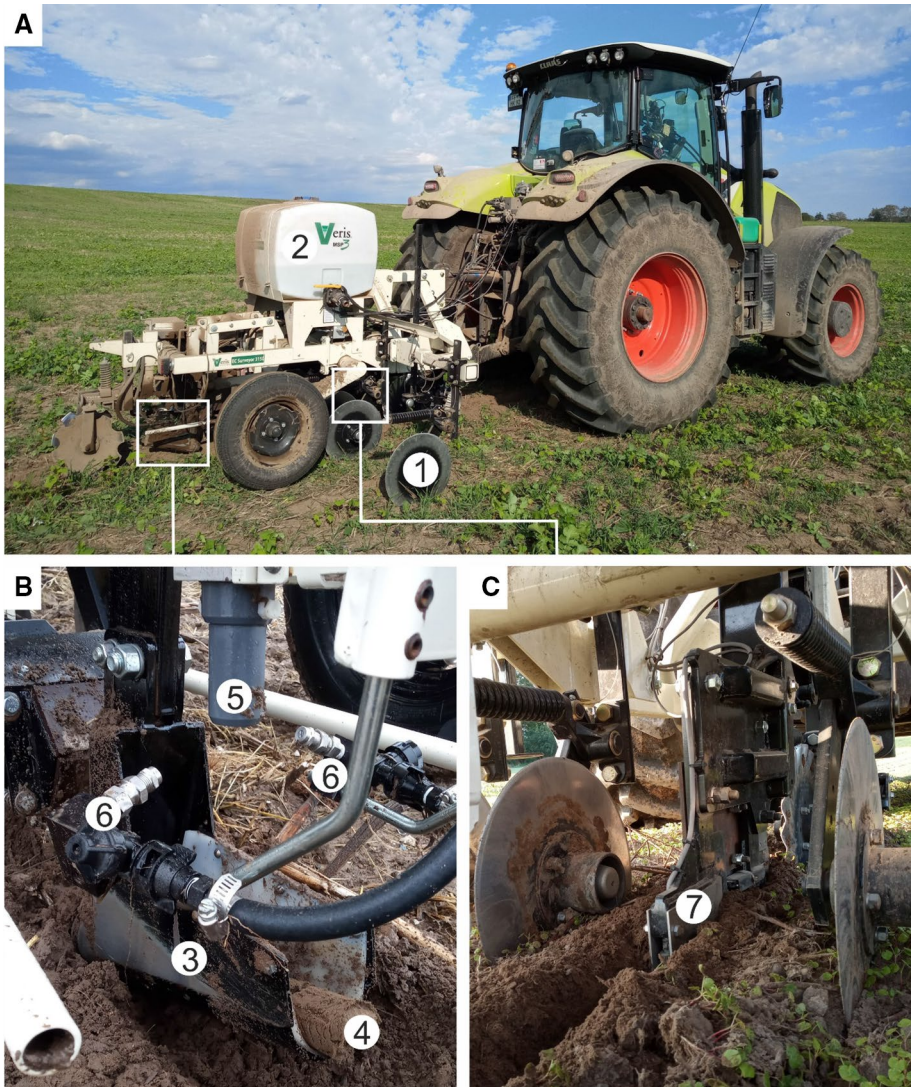
Fig. 2 A Mobile Sensor Platform (MSP) developed and manufactured by Veris Technologies™ (Salinas, KS, USA) with ECa instrument (1), B soil pH Manager (water tank (2), soil sampler (3) with sample (4), pH electrodes (5), and cleaning nozzles (6), and C OpticMapper with and optical module (7) in between the ECA coulter electrodes (photos: Torsten Schubert)
