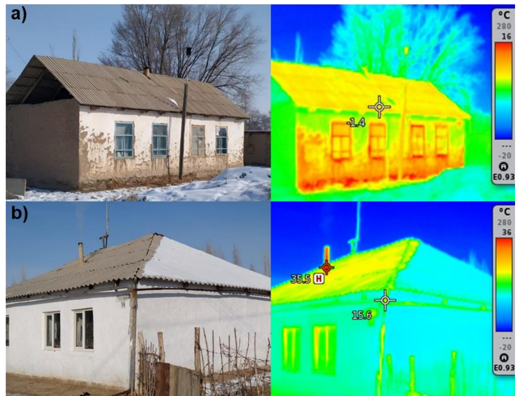
Figure 8. Thermal images of different Kyrgyz houses in the Ak-Tal region during the heating season (February 2020) (a) the old and uninsulated building, (b) newly built house [source: author].
