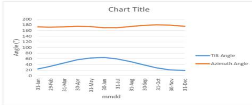
Figure 17 Tilt and azimuth angles change in one year
