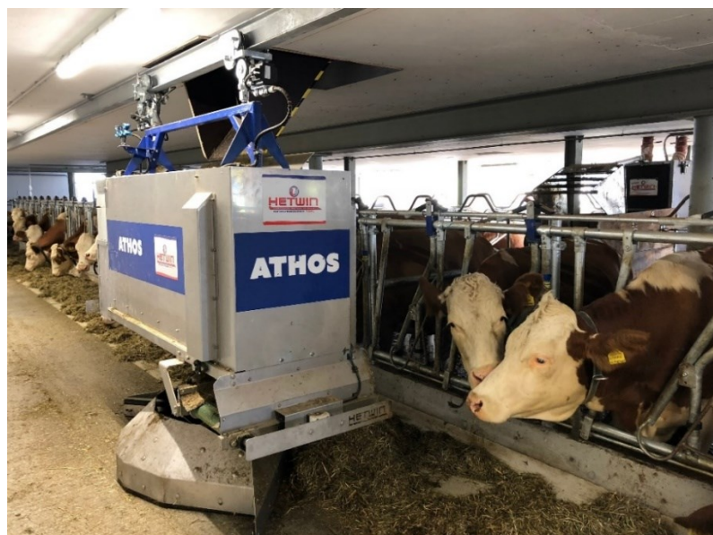
Fig 2.16: A rail-mounted AFS in a Dairy farm [47]
