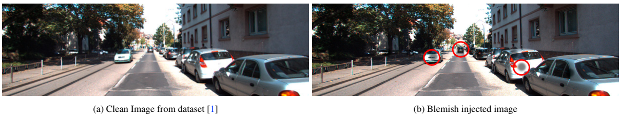
Fig. 4: Example of synthetic blemishes, inserted onto a clean image at known positions of objects.
