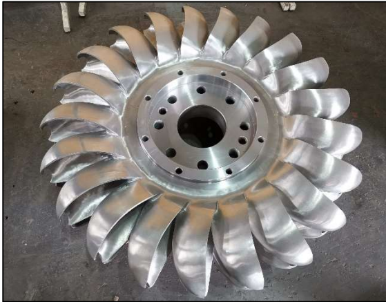
Figure 19: Casted Pelton turbine [saVRee, 2020]
