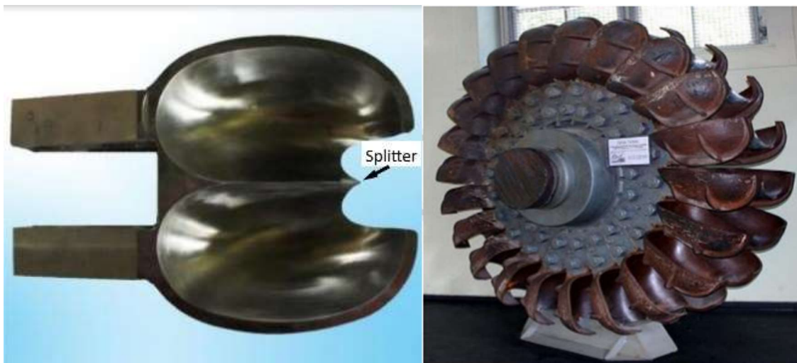
Figure 11: Pelton Bucket (Left) and Pelton runner with buckets bolted (Right) [Mane M., 2020]
