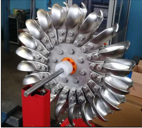
Figure 18: Bolted Pelton buckets on runner. [Guglielmi Alessandro, 2020]
