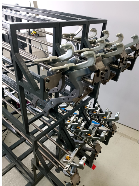
Figure 14: Partial flowrack with few hinges
