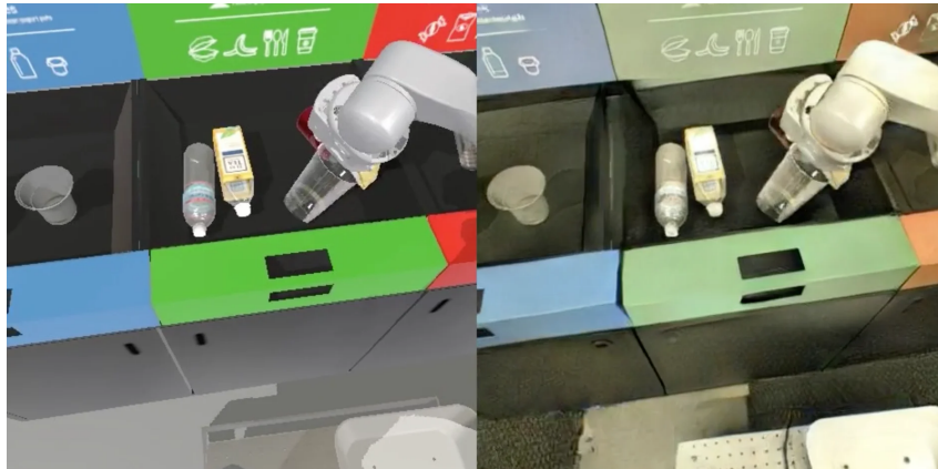
Figure 8: Sim2Real gap - Simulated (left) vs real (right) image [20]
