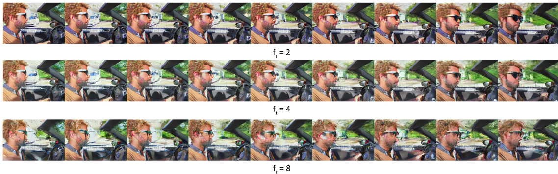
Figure 4: Visual comparison between different temporal compression ratios f_t \in [2, 4, 8] . More compression leads to worse reconstructions spatially and temporally.
