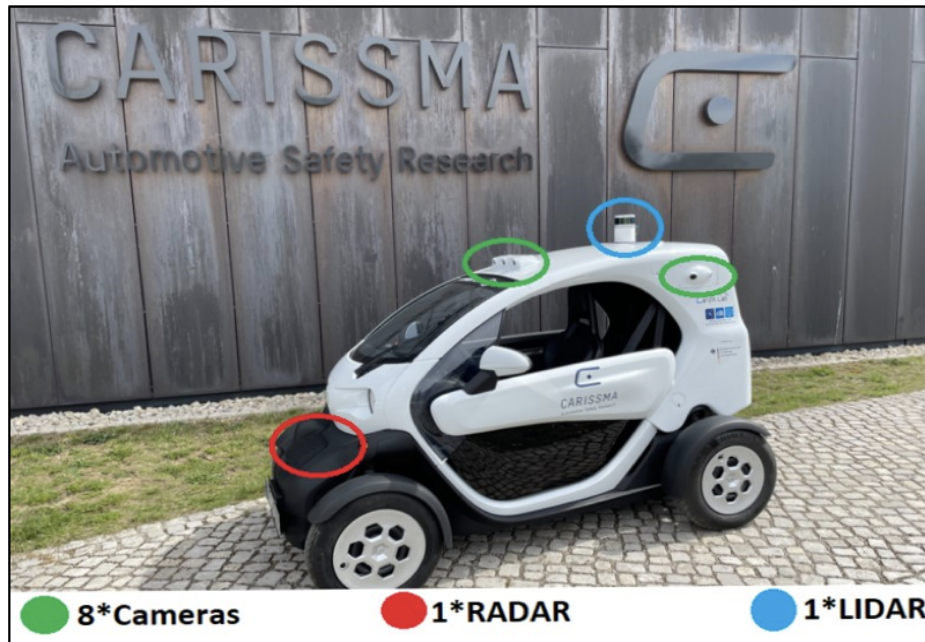
Figure 1.2: Autonomous Vehicle ANTON with highlighted LIDAR, RADAR, and Camera Sensors [4]
