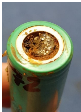
Figure 3. Incrustations at the positive terminal of the cell for TW for two weeks.
