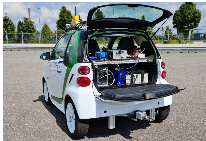
Figure 2. Test vehicle equipped with (1) an ADMA in the trunk (blue), (2) a Correvit sensor on the trailer hitch (gray), (3) a car PC in the trunk (gray), (4) a SatNav receiver on the roof (gray), and (5) a radio antenna for RTK correction data on the roof (black).
