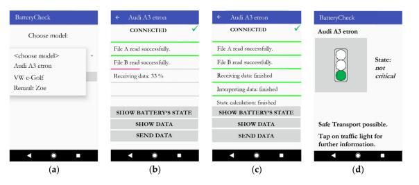
**Figure 5.** User interface of the app "BatteryCheck" (selected example model: Audi A3 e-tron): (a) initial view with available models; (b) view while receiving data from the BMS; (c) view after successful reception and evaluation of data; (d) display of calculated safety-state result with additional information.
