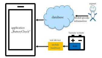
**Figure 6.** Data context of the application "BatteryCheck": Besides the data read from the battery's BMS with the mobile hardware, the application is taking model-specific information from a backend database, which includes expert knowledge needed to decode the raw CAN-data.
