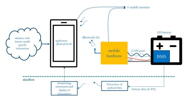
**Figure 8.** Complete conceptual overview of the mobile interface and information flow: the mobile hardware reads battery data from a BMS wire-bound, extracts the payload information and transfers it wirelessly to the application "BatteryCheck", where the data are decoded and evaluated based on model-specific information stored in a database.
