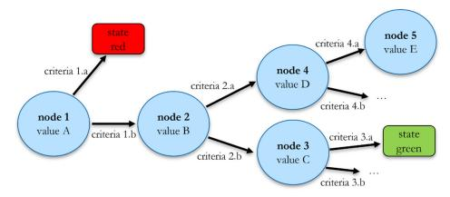
**Figure 7.** App "BatteryCheck"—assessment principle of BMS data with a decision tree: every node corresponds to a certain CAN-signal, which was received from the BMS and decoded by the application. Depending on the physical values and the defined evaluation criteria, a certain state is calculated.
