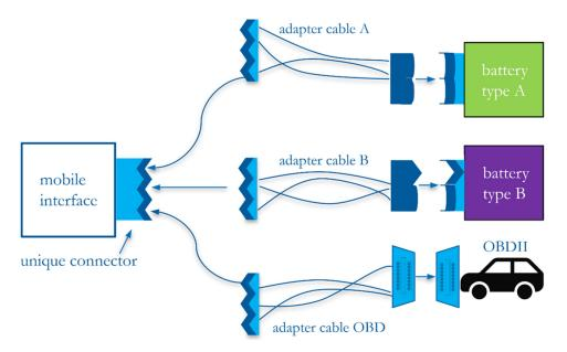
**Figure 3.** Mobile interface—concept of physical connection: with respective adapter cables, the mobile interface can be universally applied to a variety of battery models as well as directly connected to the OBDII port.
