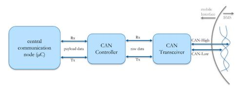
**Figure 4.** Physical data connection to BMS channel: data that are sent on the CAN-H and CAN-L line of the BMS are read into the CAN-Transceiver and forwarded to the CAN-Controller, which extracts the payload data from the complete data stream to be input into the microcontroller.
