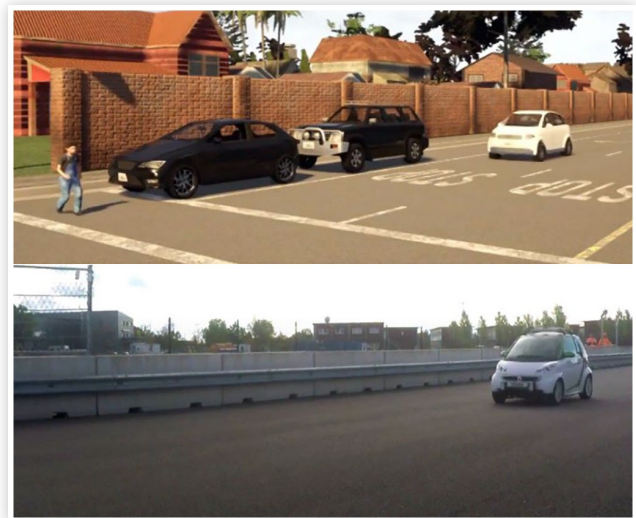
FIGURE 1 Virtual surroundings created in the simulation (top) and DynViL on the empty test track (bottom).
