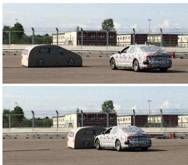
Figure 1. Crash test with dummy vehicle on the CARISSMA outdoor facility at Technische Hochschule Ingolstadt
