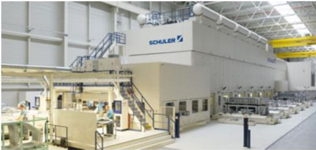
Figure 2.12: Servo press line with blank holder and crossbar feeder, Metal Forming Handbook, Schuler GmbH [40]
