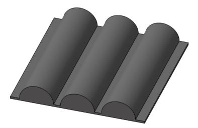
**Figure 6.** Crush plate for module as per UN/ECE-R100.02:2013 [98], GTR 20:2018 [108], SAE J2464:2009 [89], ISO 12405-3:2014 [84], and FreedomCAR:2006 [92].
