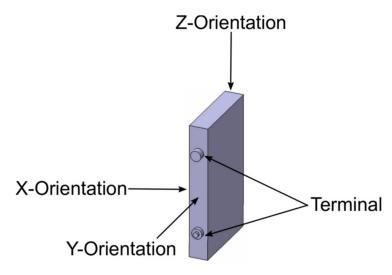
Figure 4. X-, Y- and Z-orientation of prismatic cell as per SAND2017-6925:2017 [107].
