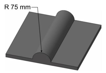
Figure 7. Crush plate for the module as per SAND2017-6925:2017 [107].
