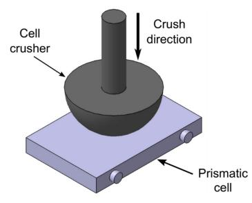
Figure 9. Cell crusher for prismatic cells as per IEC 62660-2:2010 [87].
