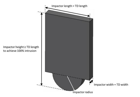
Figure 10. Impactor for crushing prismatic and pouch cell as per SAND2017-6925:2017 [107].
