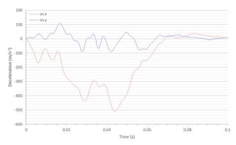
**Figure 12.** Decelerations during a crash test (speed: 54 km/h, rigid barrier, full overlap, 0° impact angle) [121].
