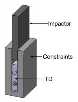
**Figure 5.** Prismatic cell in the fixture and crushed along Z-orientation as per SAND2017-6925:2017 [107].
