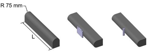
Figure 2. Cell crush board as per GB/T 31485-2015:2015 [40].
